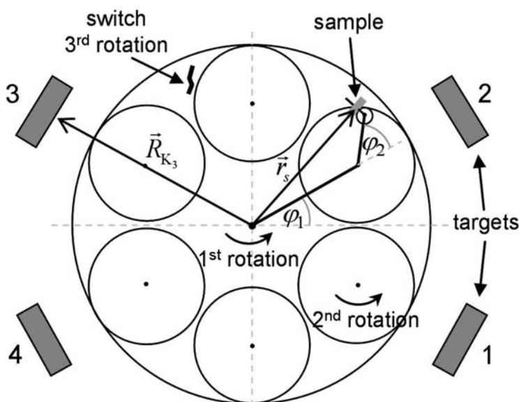
**Figure 1.** Schematic top view of the CC800/9 (CemeCon)
