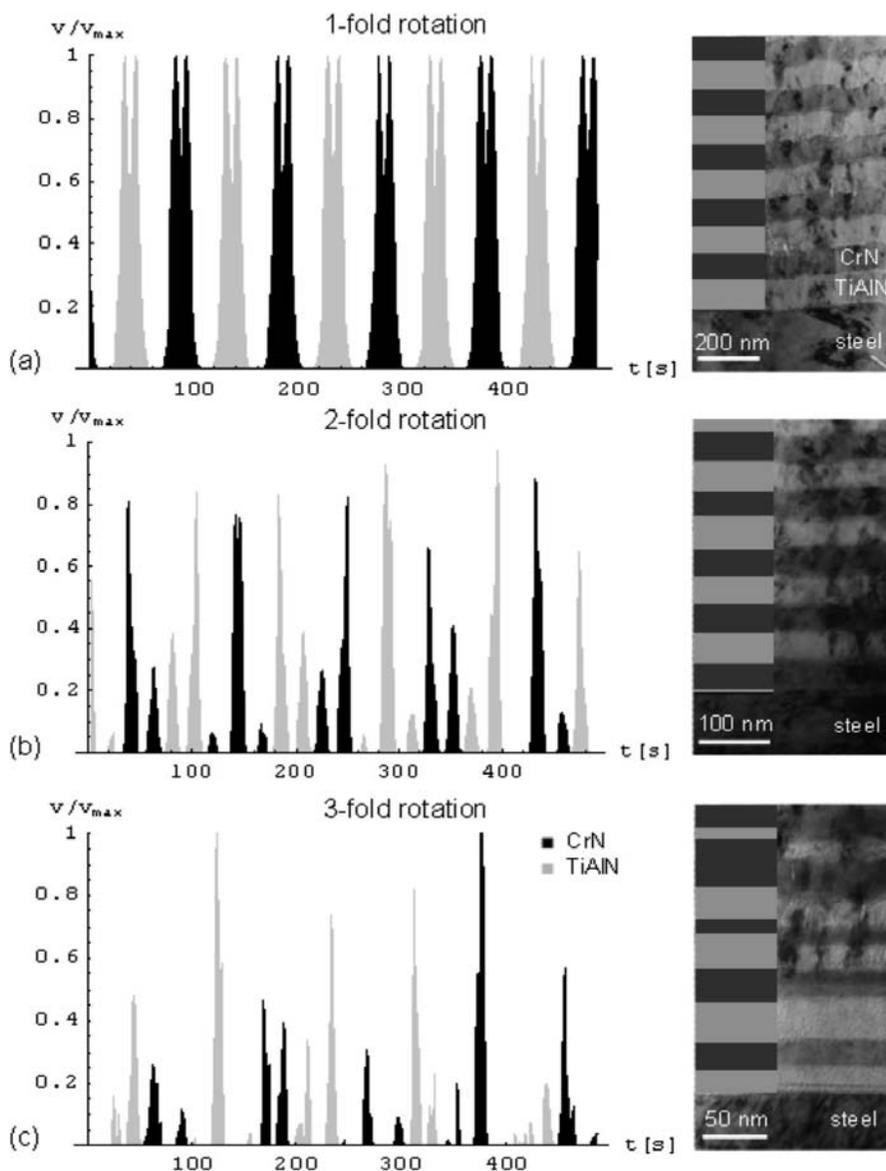
**Figure 5.** The deposition rate and the layer structure for (a) 1-, (b) 2-, and (c) 3-fold rotation. Calculated layered structures are compared to the TEM micrographs of the deposited TiAlN/CrN nanolayered coatings<sup>[10]</sup>
