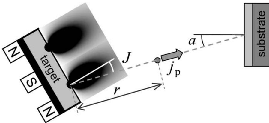
Figure 2. Particle flux from the magnetron target
