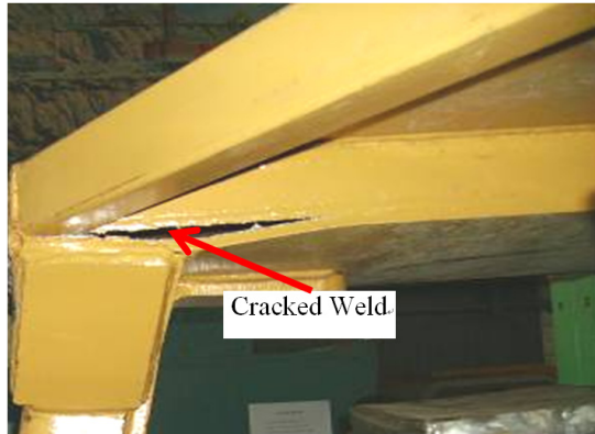
Fig. 2. Cracking failure of weld in two-post ROPS connection
