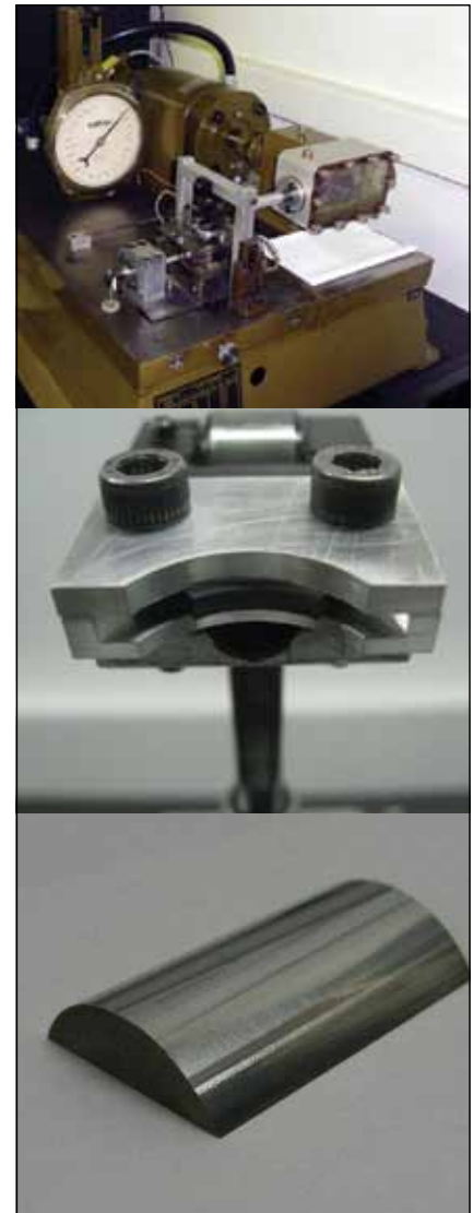
Figure 6. Tribological test rig with measurement accessories
