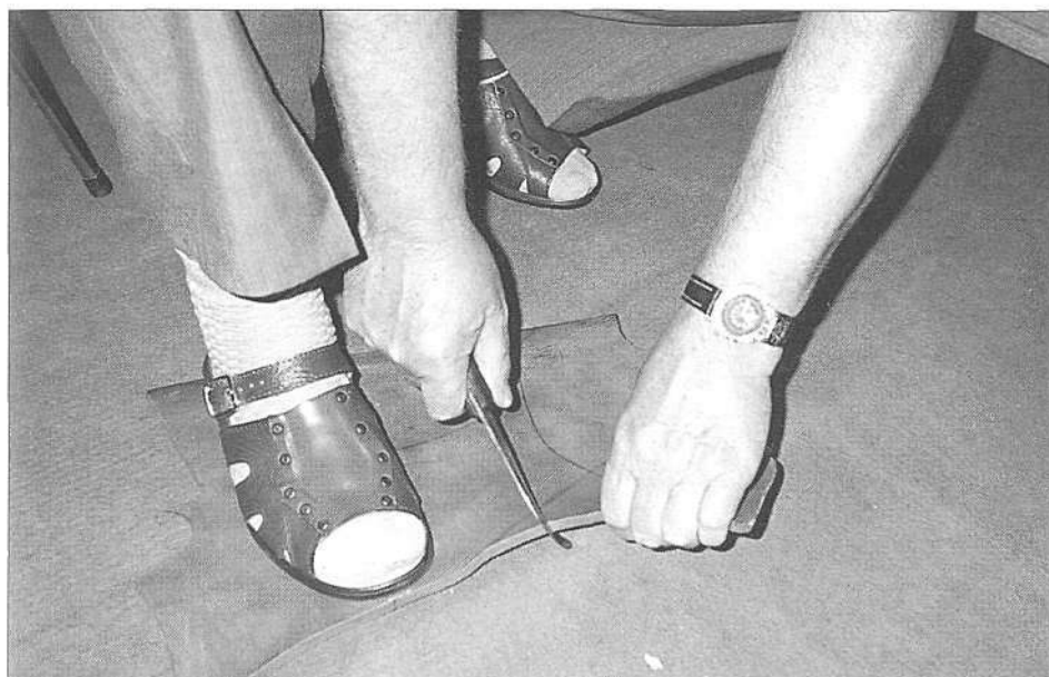
Rezanje karpona s krivcem (foto Tita Ovsenar, fototeka Tržiškega muzeja, inv. št. 727). ♦ Cutting sole-leather with a shoemaker's knife (photo Tita Ovsenar, picture library of the Tržič Museum, inv. no. 727).
