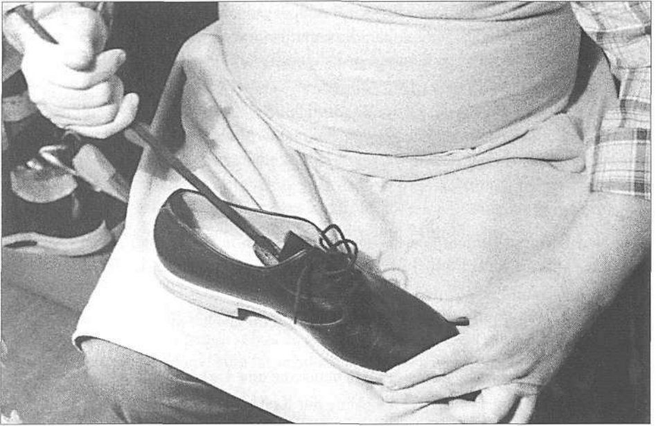
Ostrgovanje lesenih cvekov v čevlju, uporaba strgala – auskrocjarja (foto Alenka Krašovec, fototeka Tržiškega muzeja, inv. št. 1521). ♦ Scraping off wooden nails in a shoe, how a scraper is used (photo Alenka Krašovec, picture library of the Tržič Museum, inv. no. 1521).
