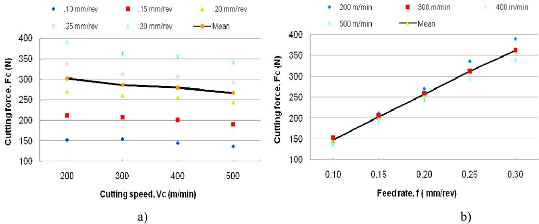
Fig. 6. Main cutting force values for AA2014 (T4) alloy determined during machining with uncoated carbide cutting tool: a) depending on cutting speed, b) depending on feed rate
