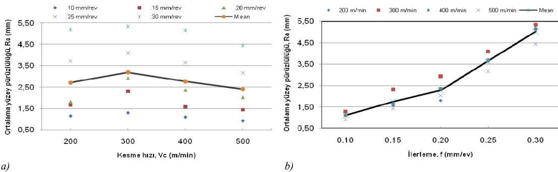
Fig. 7. Average surface roughness ( $R_a$ ) values for AA2014 (T4) alloy determined during machining with uncoated carbide cutting tool: a) depending on cutting speed, b) depending on feed rate
