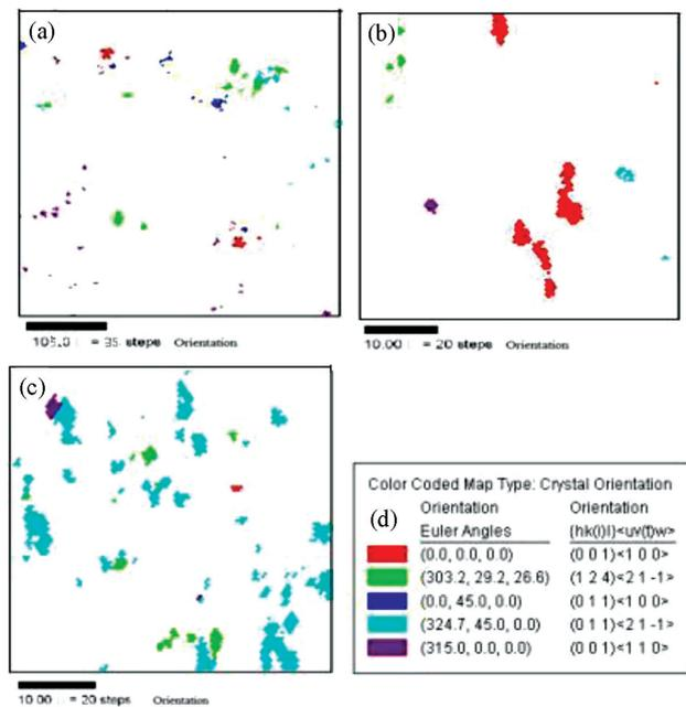
**Figure 6:** Texture distribution of rolled 1235 aluminum alloy for: a) 50-% hot rolling, b) 90-% hot rolling, c) 90-% cold rolling, d) color-coded map
