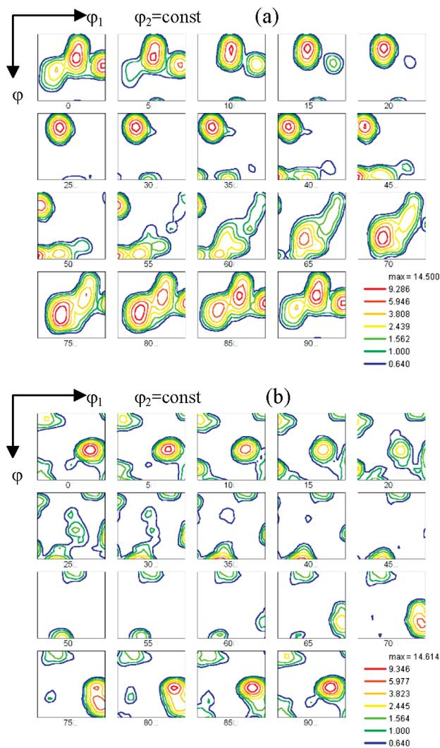
**Figure 1:** ODF of 1235 aluminum alloy after hot rolling: a) 50-% hot rolling, b) 90-% hot rolling
