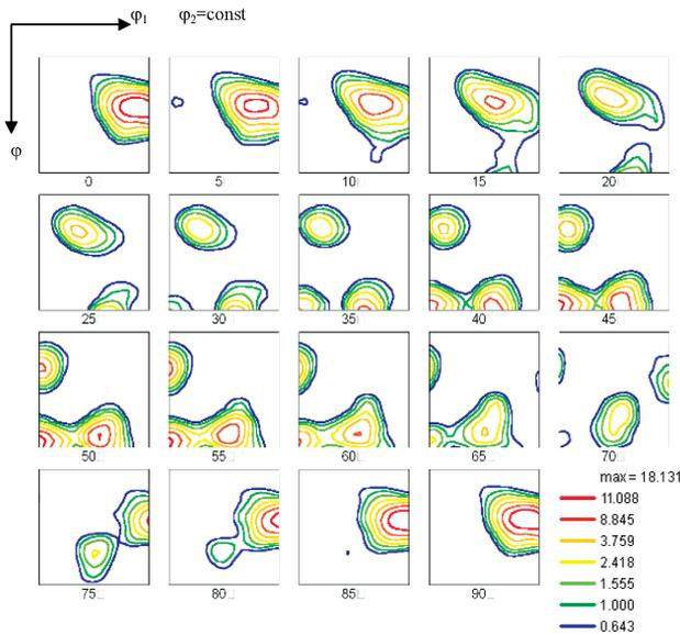
Figure 3: ODF of 90-% cold-rolled 1235 aluminum alloy
