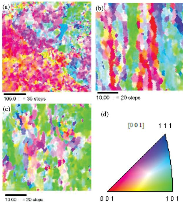
**Figure 5:** Grain orientation of rolled 1235 aluminum alloy for: a) 50-% hot rolling, b) 90-% hot rolling, c) 50-% cold rolling, d) IPF for orientation distribution
