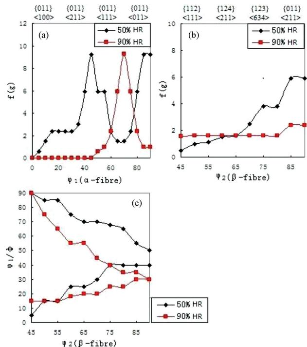
**Figure 2:** Orientation-line distribution of 1235 aluminum alloy after hot rolling (HR): a) orientation line  $\alpha$ , b) orientation line  $\beta$ , c) location of orientation line  $\beta$  in the orientation space
