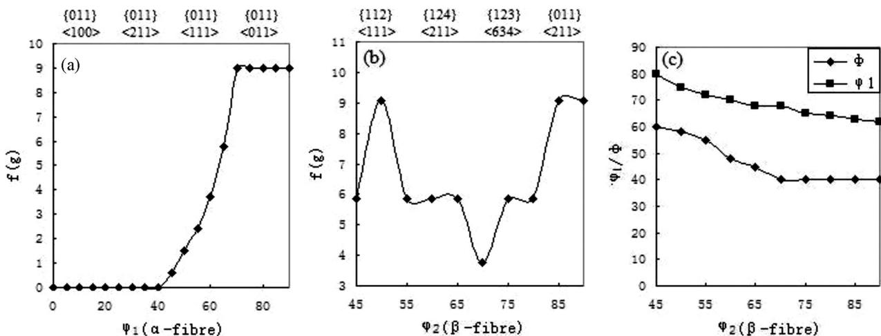
Figure 4: Orientation-line distribution of 90-% cold-rolled 1235 aluminum alloy for: a) orientation line  $\alpha$ , b) orientation line  $\beta$ , c) location of orientation line  $\beta$  in the orientation space
