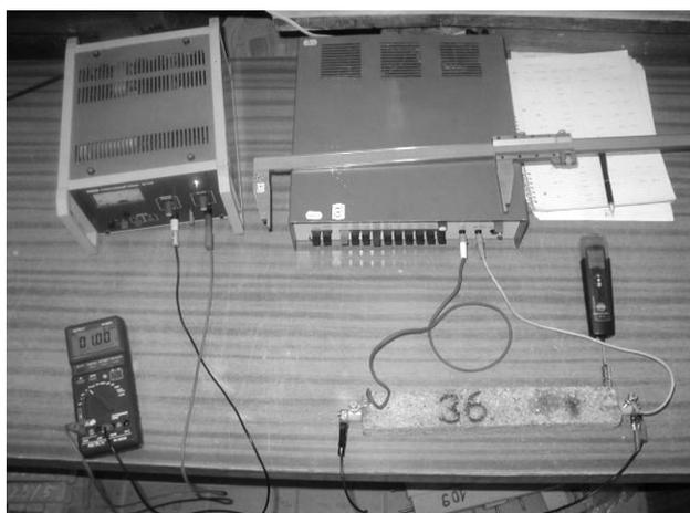
**Figure 3:** MER of embedded steel bars using a set of apparatus
