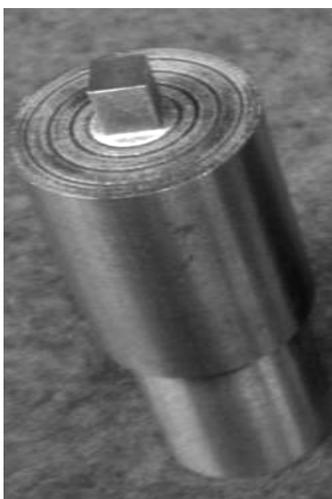
**Figure 1:** Photograph of manufactured FSW tool
