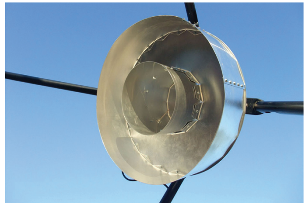
Figure 4: Practical implementation of the VE4MA feed.
