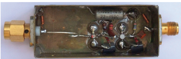
Figure 8: Practical implementation of the LNA.
