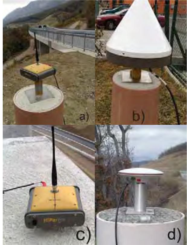
Figure 5. a-d: Different types of antennas and receivers.
