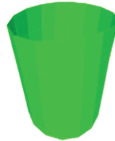
Figure 12: 2 nd mode shape ( f = 8.33 Hz, \xi = 0.85 )
