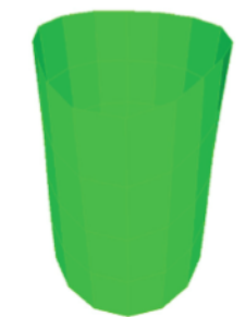
Figure 9: 5 th mode shape ( f = 11.87 Hz, \xi = 0.64 )
