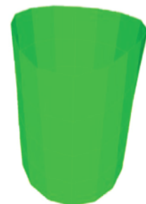
Figure 15: 5 th mode shape ( f = 14.46 Hz, \xi = 0.54 )
