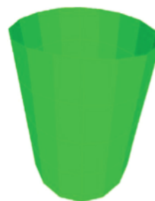
Figure 5: 1 st mode shape ( f = 5.45 Hz, \xi = 1.04 )
