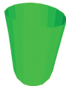
Figure 6: 2 nd mode shape ( f = 7.32 Hz, \xi = 0.88 )
