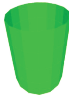
Figure 13: 3 rd mode shape ( f = 11.25 Hz, \xi = 0.62 )
