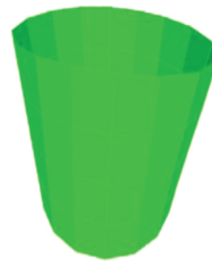
Figure 11: 1 st mode shape ( f = 6.10 Hz, \xi = 0.97 )
