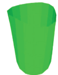
Figure 8: 4 th mode shape ( f = 10.63 Hz, \xi = 0.82 )
