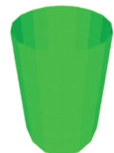
Figure 7: 3 rd mode shape ( f = 9.87 Hz, \xi = 0.71 )
