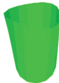
Figure 14: 4 th mode shape ( f = 12.78 Hz, \xi = 0.73 )
