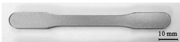
Figure 2: General view of tensile test specimen sintered at 1350 °C for 1 h
