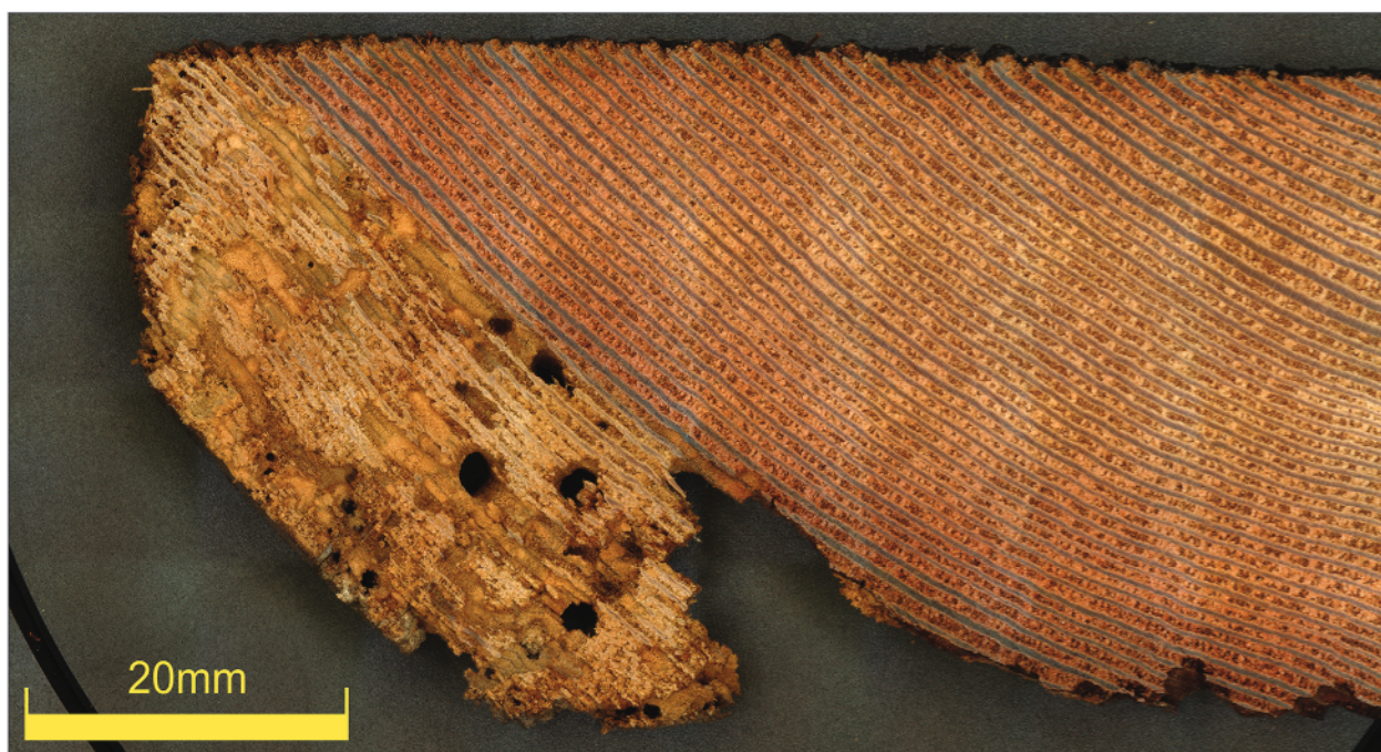
Slika 4. Prečni prerez vzorca macesna iz Ruardove graščine z beljavo, ki so jo poškodovali insekti Figure 4. Cross-section of a larch sample from Ruard's mansion with the sapwood damaged by insects
