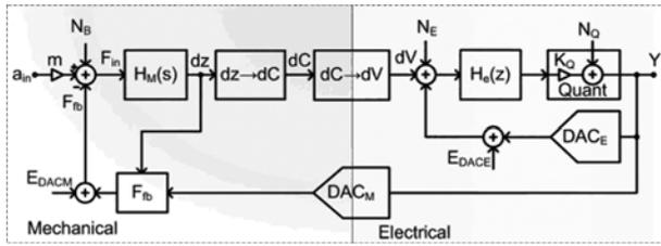
**Figure 1:** Generic electromechanical  $\Sigma\Delta$  modulator
