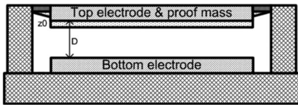
**Figure 2:** MEMS sensor
