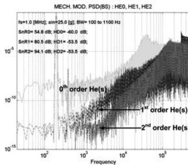
**Figure 6:** Spectrums of three MEMS  $\Sigma\Delta$  modulators with different orders of electronic noise shaping filters.
