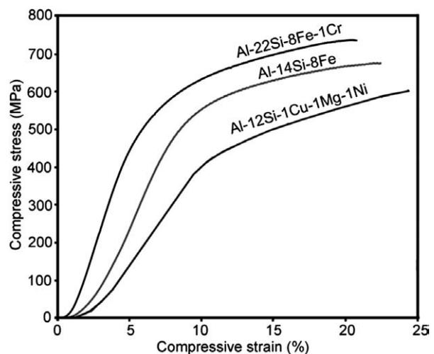
**Figure 6:** Compressive stress-strain diagrams of the investigated alloys
