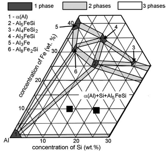
**Figure 5:** Aluminium corner of the Al-Si-Fe phase diagram<sup>4</sup> (the chemical compositions of the investigated P/M alloys are marked with black cubes)
