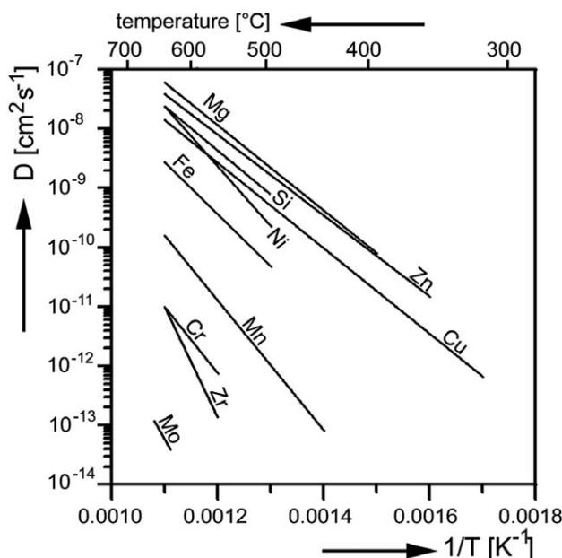
Figure 9: Arrhenius plots of diffusion coefficients  $D_s$  of various metals in Al.<sup>7</sup> Transition metals like Fe have significantly lower diffusion coefficients than the commonly used alloying elements like Cu, Si or Mg.
