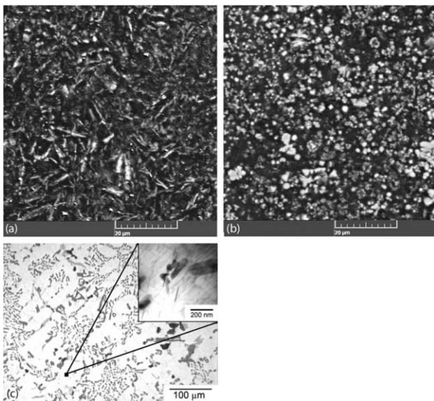
**Figure 4:** Microstructures of the investigated alloys: a) the PM Al-14Si-8Fe alloy (SEM), b) the PM Al-22Si-8Fe-1Cr alloy (SEM), c) the casting Al-12Si-1Cu-1Mg-1Ni (T6) alloy (LM, TEM)
