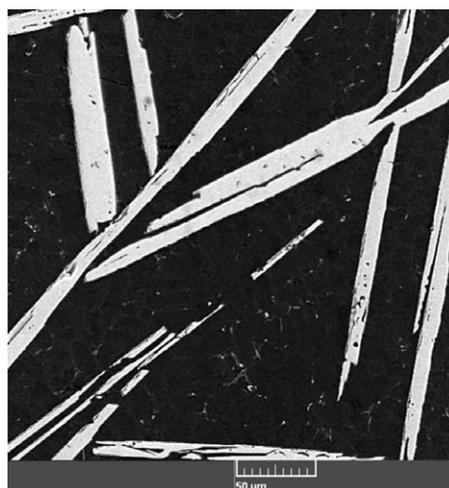
**Figure 1:** SEM micrograph of the as-cast Al-14Si-8Fe alloy containing large  $\beta$ -Al<sub>5</sub>FeSi plates (light) deteriorating the mechanical properties
