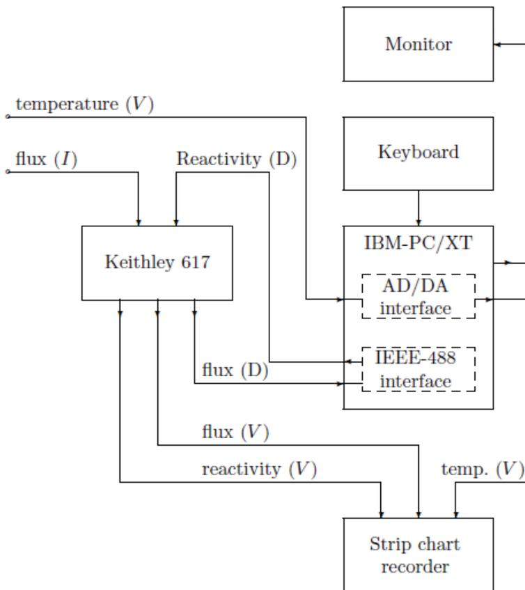
**Figure 2:** Block diagram representing the digital reactivity meter DMR-043 hardware connections. ( $D$ ) represents a digital signal, ( $V$ ) represents an analogue voltage signal, and ( $I$ ) represents an analogue current signal, [4]
