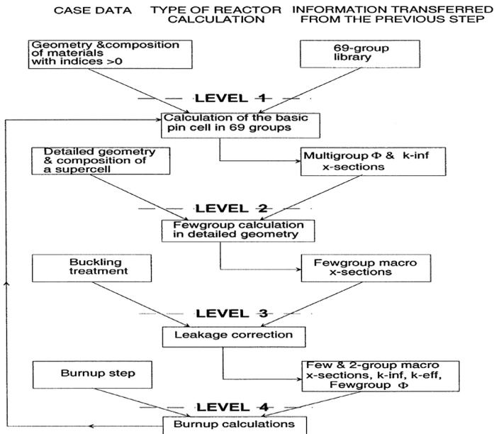
Figure 3: Simplified flowchart of the WIMS-D calculations, [2]
