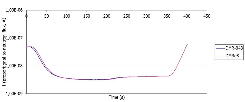
**Figure 7:** Time-variation of the neutron flux measured in the TRIGA reactor
