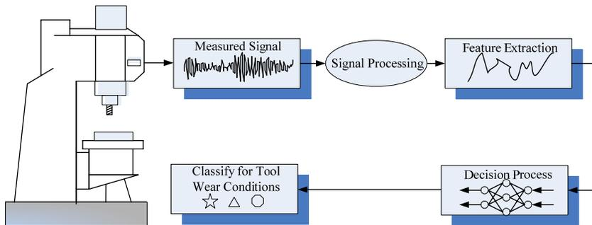
Fig. 1. *Recognition process for monitoring tool wear*
