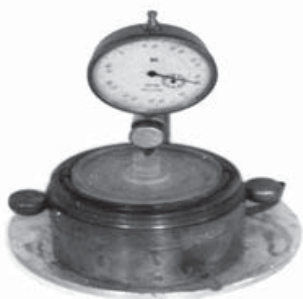
Figure 2. Test of inflation in a free cell oedometer (without piston).
