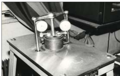
Figure 3. Swelling test in an oedometer under load.
