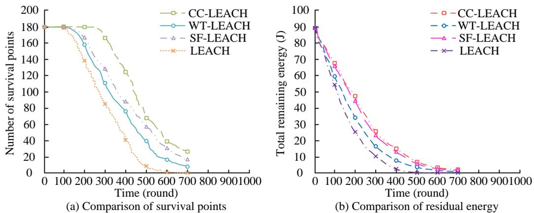
Figure 8: Comparison of the surviving nodes and remaining energy results in different algorithms
