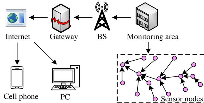
Figure 2: Schematic diagram of WSN architecture
