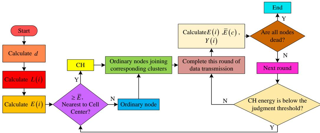
Figure 3: CC-LEACH algorithm process
