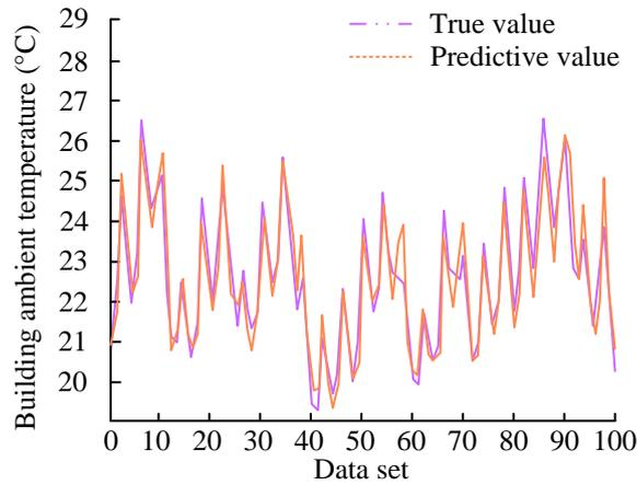
Figure 10: Comparison of real and predicted values of building environment
