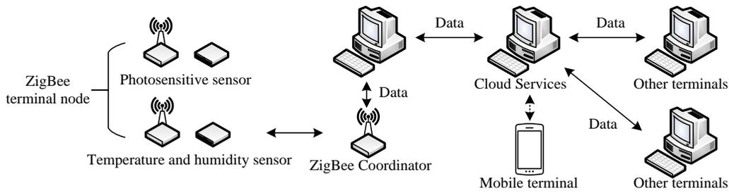
Figure 5: Schematic diagram of Zigbee system
