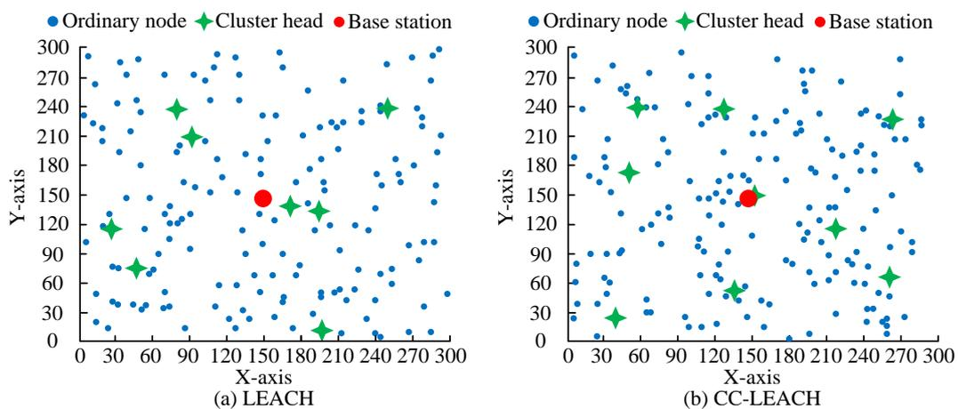
Figure 7: Comparison of CH distribution between LEACH and CC-LEACH in WSN
