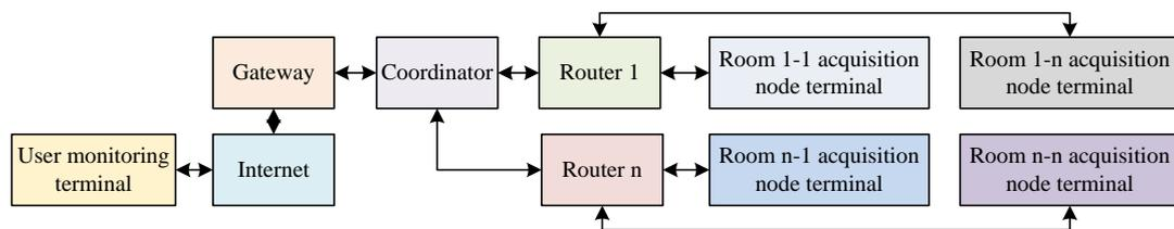
Figure 4: Schematic diagram of the overall system architecture
