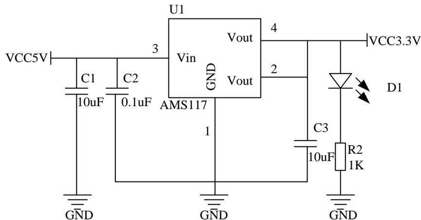
Figure 6: Schematic diagram of the power supply circuit
