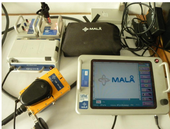
Figure 4.3: The radar system used for the GPR measurements.
