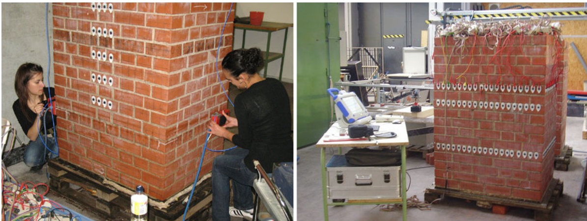
Fig. 3 Radar tomographic measurement over cross section A–A and CR tomographic measurement over several cross sections using the LGM device
