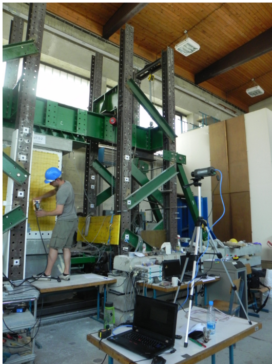
Fig. 3. GPR and IR thermography test set-up.
