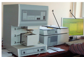
Fig. 5. The Netzsch DMA 242 C principle of measurement
