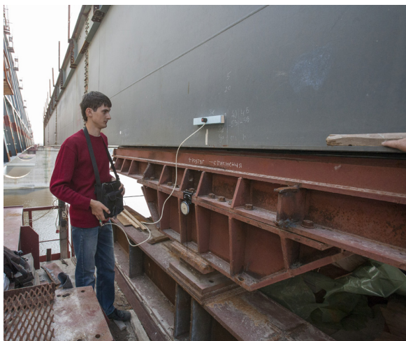
Fig. 14. The measurement of stress changes in the bridge framework sidewall at the time of the launching
