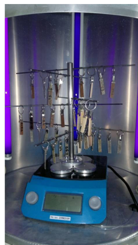
Fig. 6. Accelerated artificial weathering by UV radiations generated by UV fluorescent lamps
