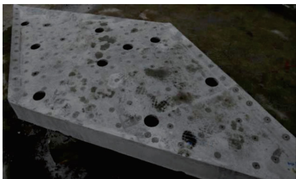
Fig. 8. Positions of core samples
