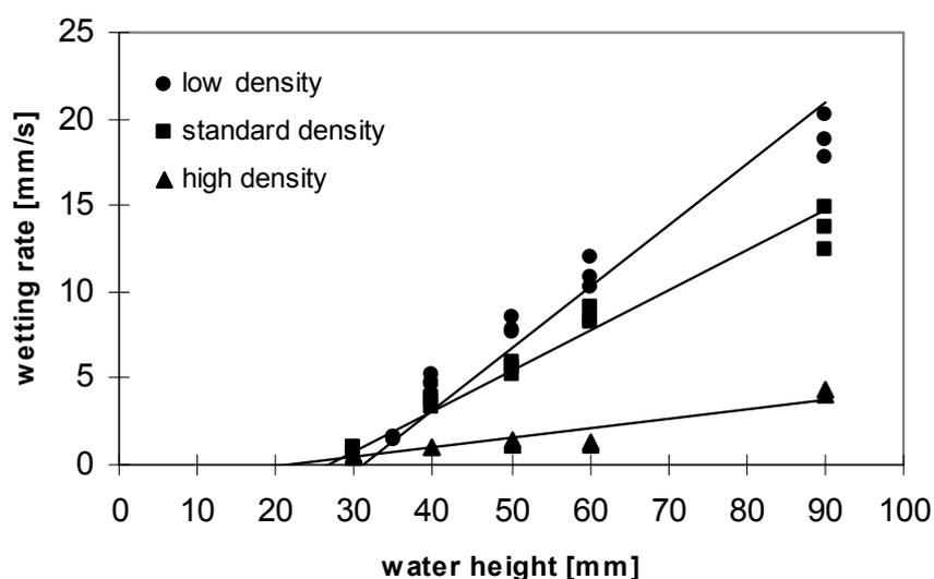
Figure 4. Wetting rate for different samples at different water heights.
