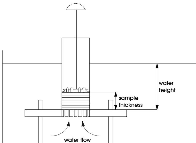
Figure 3. Schematic diagram of the wetting time measuring device.
