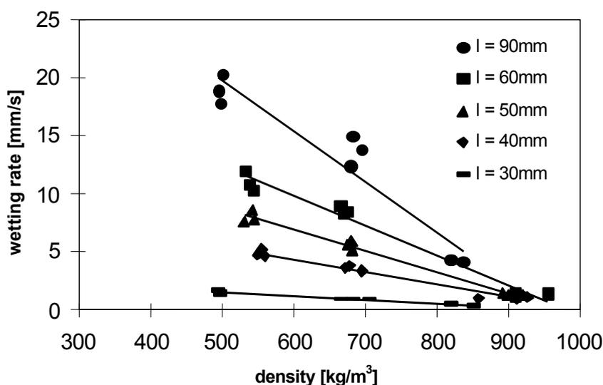
Figure 5. Wetting rate at different water depths as a function of sample density.
