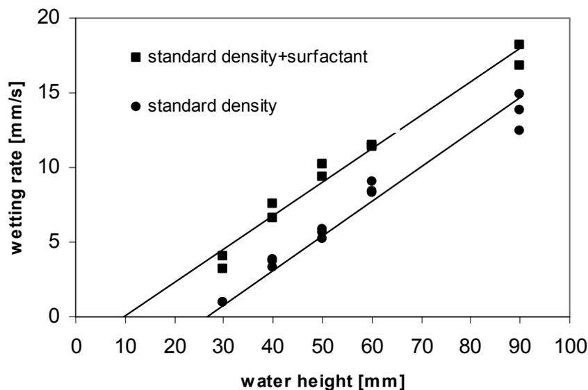
Figure 7. Effect of surfactant on wetting rate for standard density sample.
