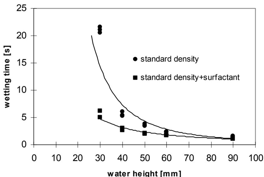
Figure 6. Effect of surfactant on wetting time for standard density sample.
