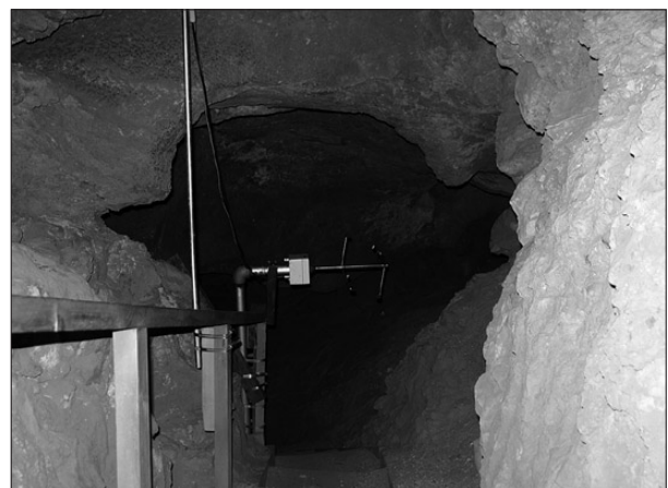
Fig. 11: Sonic anemometer in the Historic Entrance Area of Jewel Cave, South Dakota (USA) (Photo: A. Pflitsch).
