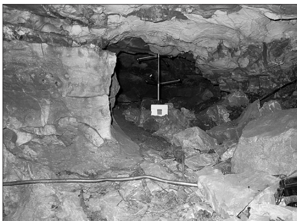
Fig. 10: Sonic anemometer in the Natural Entrance Area of Wind Cave, South Dakota (USA) (Photo: A. Pflitsch).
