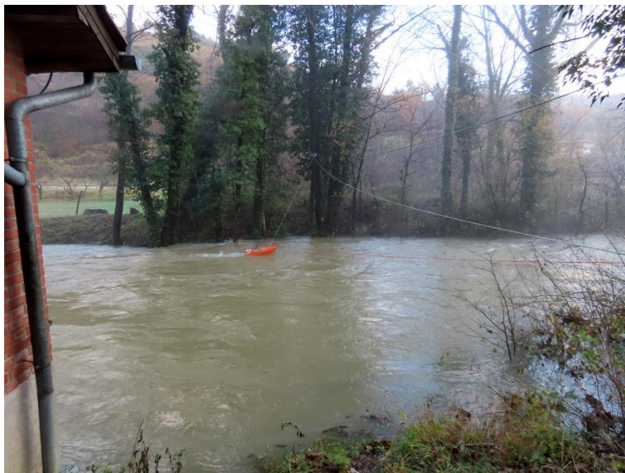
Slika 2. Meritve visokega pretoka izvira Rižane 9. decembra 2020 (foto: arhiv ARSO) Figure 2. High discharge measurement of Rižana spring on 9 th of December 2020 (photo: ARSO archive)
