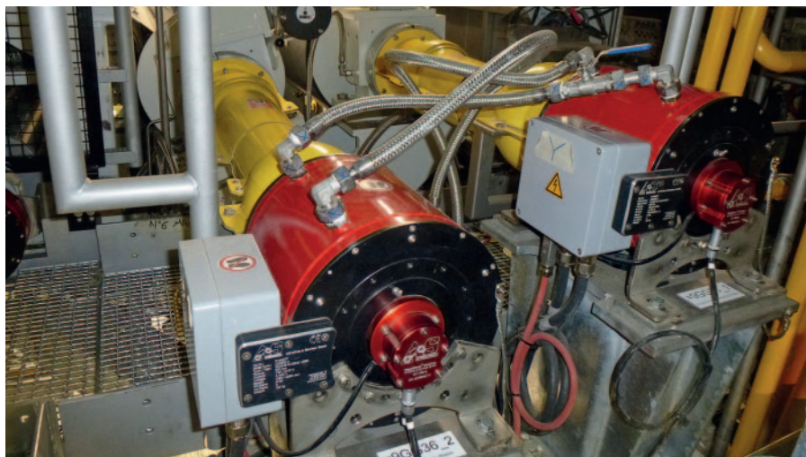
Pogon stiskalnice za globoki vlek prek FlexoDirect® / Drive of the draw press via FlexoDirect®
