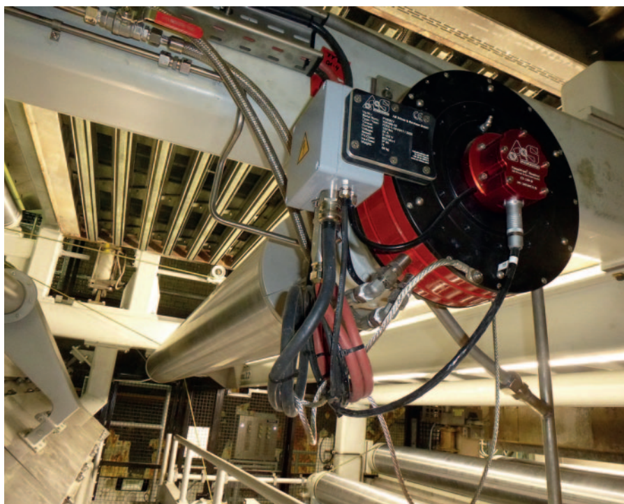
Direktni pogon FlexoDirect® kot pogon vodilnega valja / FlexoDirect® direct drive as guide roll drive
