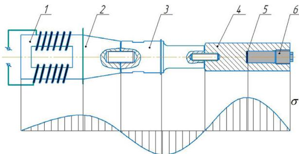
**Figure 4:** Scheme of ultrasonic processing of UFG samples in the disc form: 1 – ultrasonic transducer, 2 – concentrator, 3 – booster, 4 – waveguide, 5 – sample, 6 – preload screw
