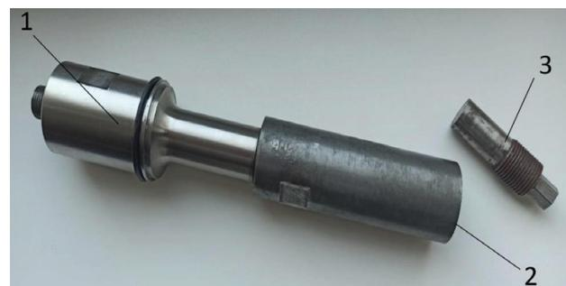
**Figure 2:** General view of the acoustic-system elements: 1 – booster, 2 – waveguide, 3 – clamping screw
