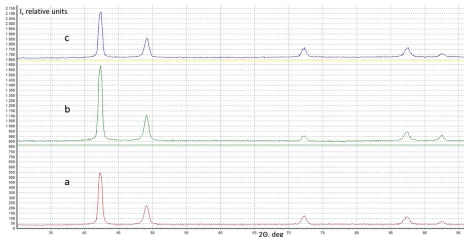
**Figure 7:** Diffractogram (CuK $\alpha$ ) of the L63 brass sample after radial-shear rolling: a – without ultrasonic processing; b – ultrasonic processing at 40 MPa; c – ultrasonic processing at 70 MPa
