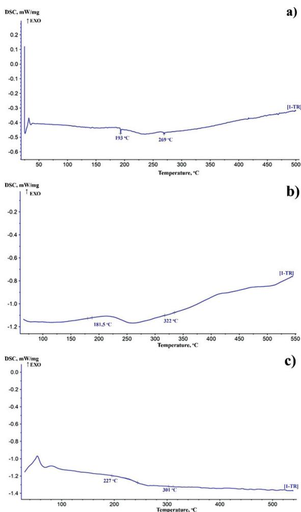
**Figure 8:** DSC curves of L63 brass samples: a – without ultrasonic processing; b – ultrasonic processing at 40 MPa; c – ultrasonic processing at 70 MPa
