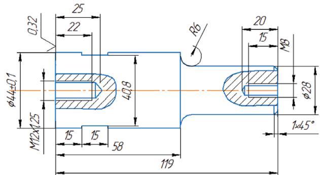
**Figure 6:** Drawing of a booster for ultrasonic processing of long samples
