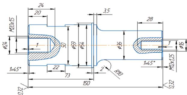
**Figure 1:** Drawing of a booster for UFG samples in the disk form
