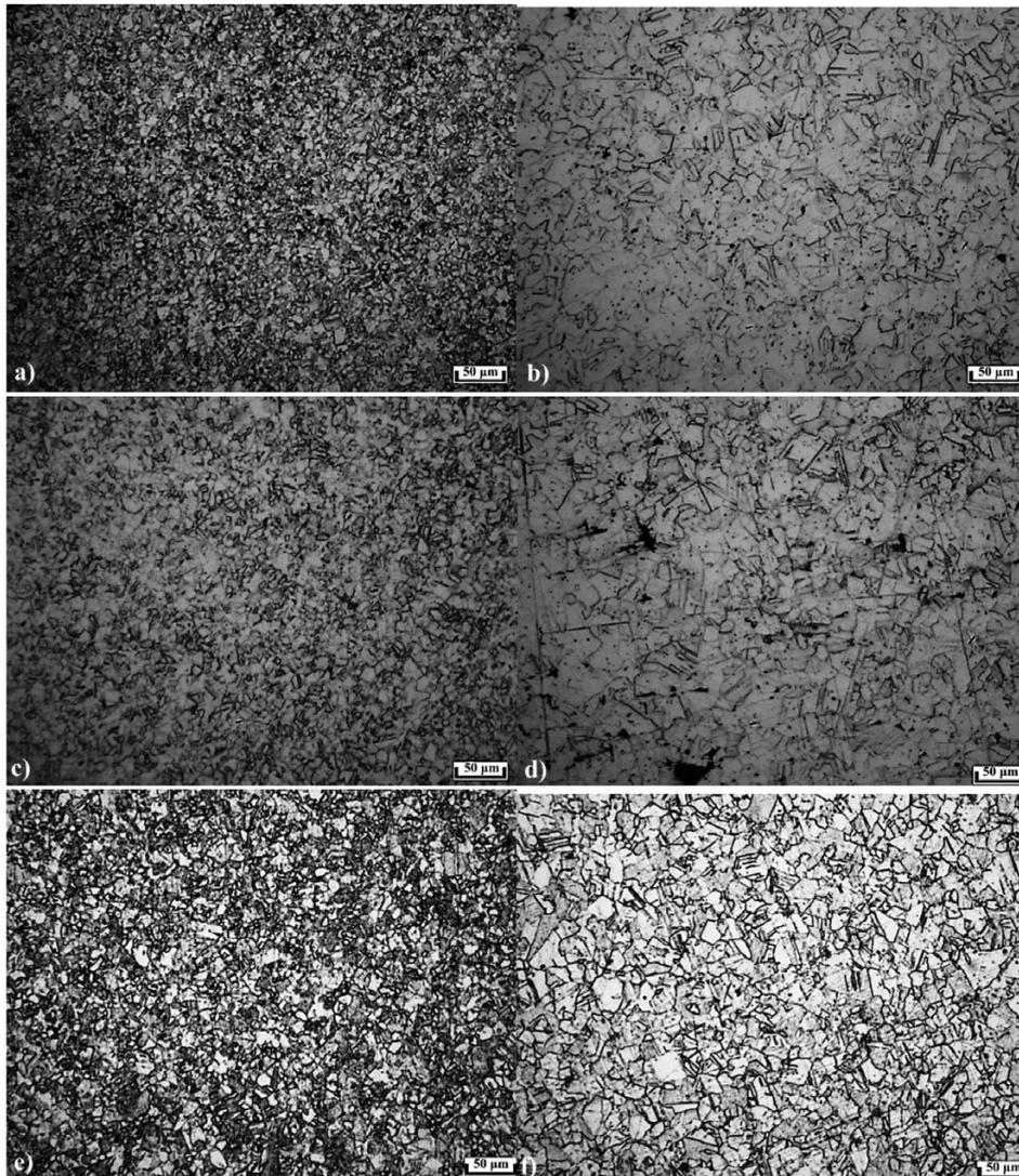
**Figure 9:** Microstructures of L63 samples at the edge of the surface (a, c, e) and in the center (b, d, f); a, b – without ultrasonic processing; c, d – ultrasonic processing at 40 MPa; e, f – ultrasonic processing at 70 MPa
