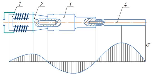
**Figure 5:** Scheme of ultrasonic processing of a long sample: 1 – ultrasonic transducer, 2 – concentrator, 3 – booster, 4 – waveguide
