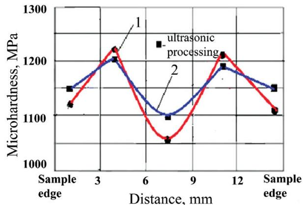
**Figure 10:** Distribution of microhardness: a) – over the diameter of a L63 disc after radial-shear rolling: 1 – without ultrasonic processing; 2 – ultrasonic processing at 40 MPa; b) – along the length of an L63 half-wave cylindrical sample after radial-shear rolling and ultrasonic processing at temperatures of: 1) 40 °C; 2) –100 °C; 3) diagram of alternating stresses at ultrasonic processing along the length of the sample
