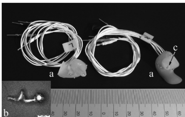
Figure 2: Plugs: a) left and right plug, b) magnified view of an electrode, c) Micro-BetaCHIP temperature probe
