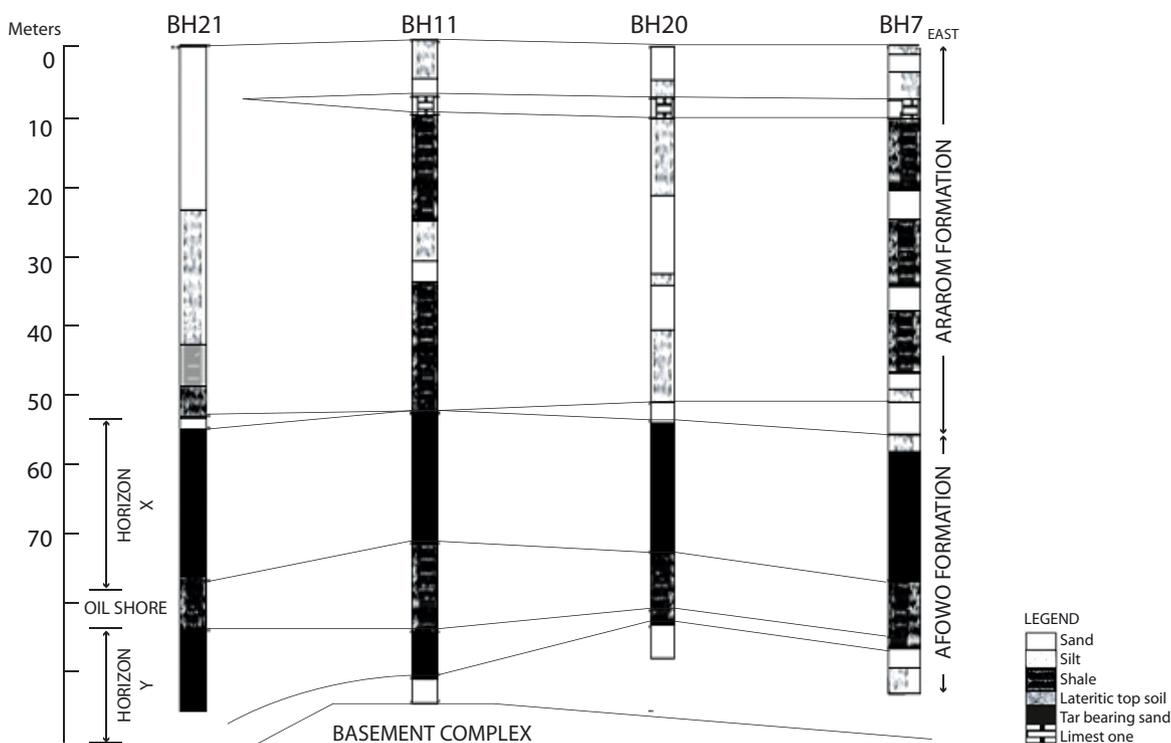
**Figure 1:** Schematic geological east-west cross-section based on drillholes showing the stratigraphic position of horizon containing tar sands horizons in some boreholes (modified from Ekweozor and Nwachukwu, 1989).
