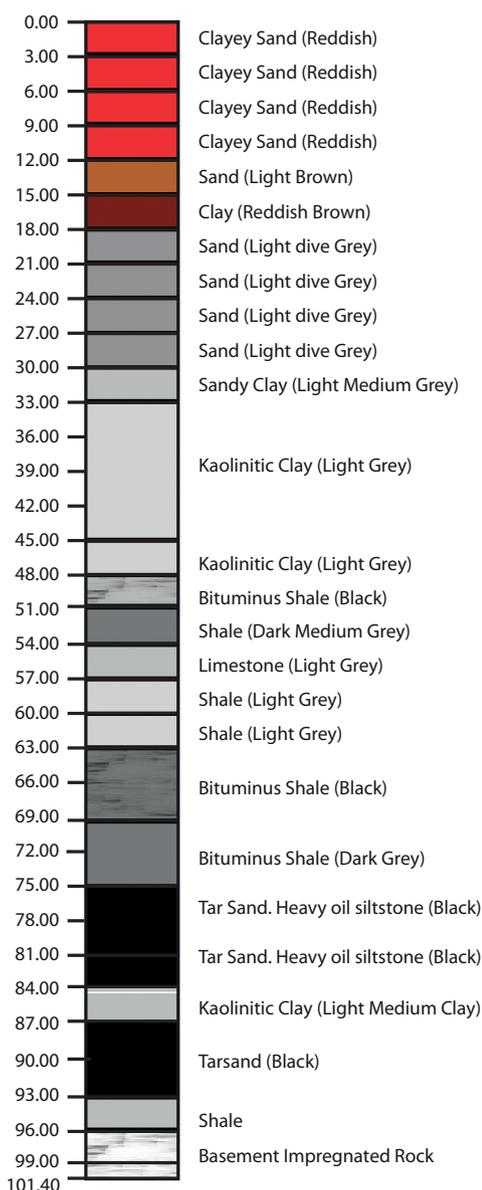
Figure 3: Lithological units of the drill hole A4.
