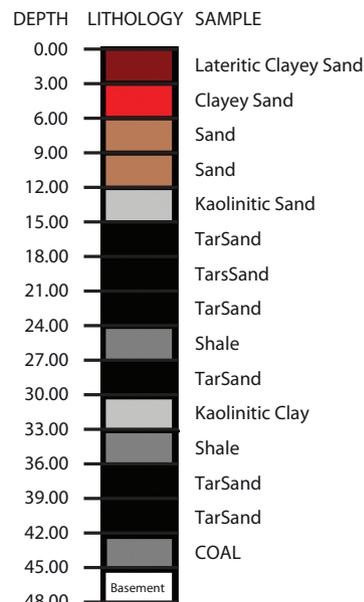
Figure 4: Lithological units of the drill hole A14.
