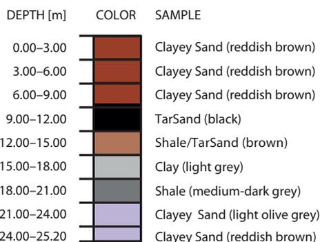
Figure 6: Lithological units of the drill hole A16.
