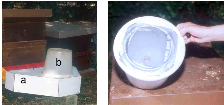
Photo 19. Left: the bee collector to sample outflying workers. The bee collector consisted of a wooden box with a wide opening at the top (a) and a plastic container (b) upside down to catch bees. Right: the plastic container to sample outflying workers. The plastic container had attached a funnel that extended its narrow part inside the container.
