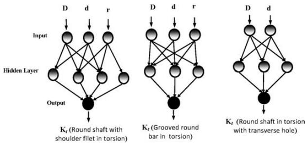
**Figure 2:** Suitable network structures for the notch factors of the shafts for: a) round shaft with a shoulder fillet in torsion, b) grooved round bar in torsion, c) round shaft with a transverse hole in torsion
