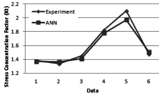
**Figure 5:** Comparison of the notch-sensitivity factors for a round shaft with a transverse hole in torsion (ANN – the actual data)
