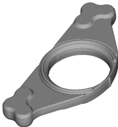
**Figure 1:** Shape of a forging – a 3D view**Slika 1:** Oblika izkovka – 3D-pogled
