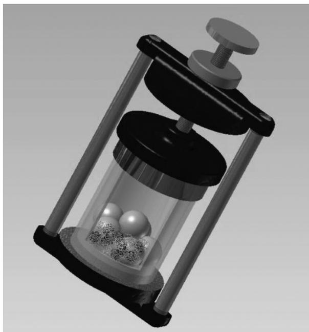
**Figure 1:** Schematic illustration of the cylindrical steel vessel placed in the holder inside the SPEX 8000 mill
