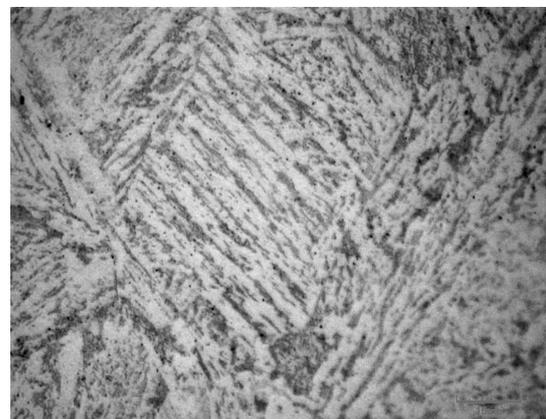
**Figure 9:** Bainite-ferrite microstructure of the forged part (HV 284)
