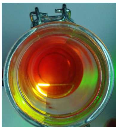
Figure 2. Directing the green laser beam to the spherical hydrogel in coloured water.
