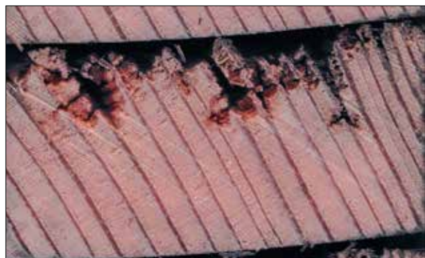
Slika 5. Presek vzorca, impregniranega z biocidnim proizvodom CCB po 14 letih izpostavitve na prostem Figure 5. Several cross-sections of wood impregnated with CCB preservative solution after 14 years of outdoor exposure
