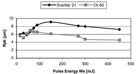
Fig. 10. Variation of  $R_{pk}$  with pulse energy,  $W_e$
