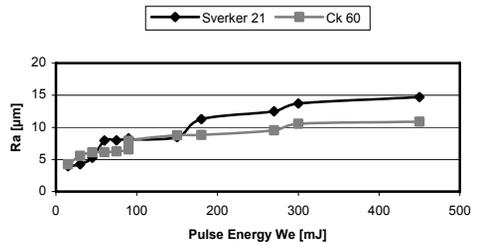
Fig. 2. Variation of average roughness *R<sub>a</sub>*, with pulse energy, *W<sub>e</sub>*
