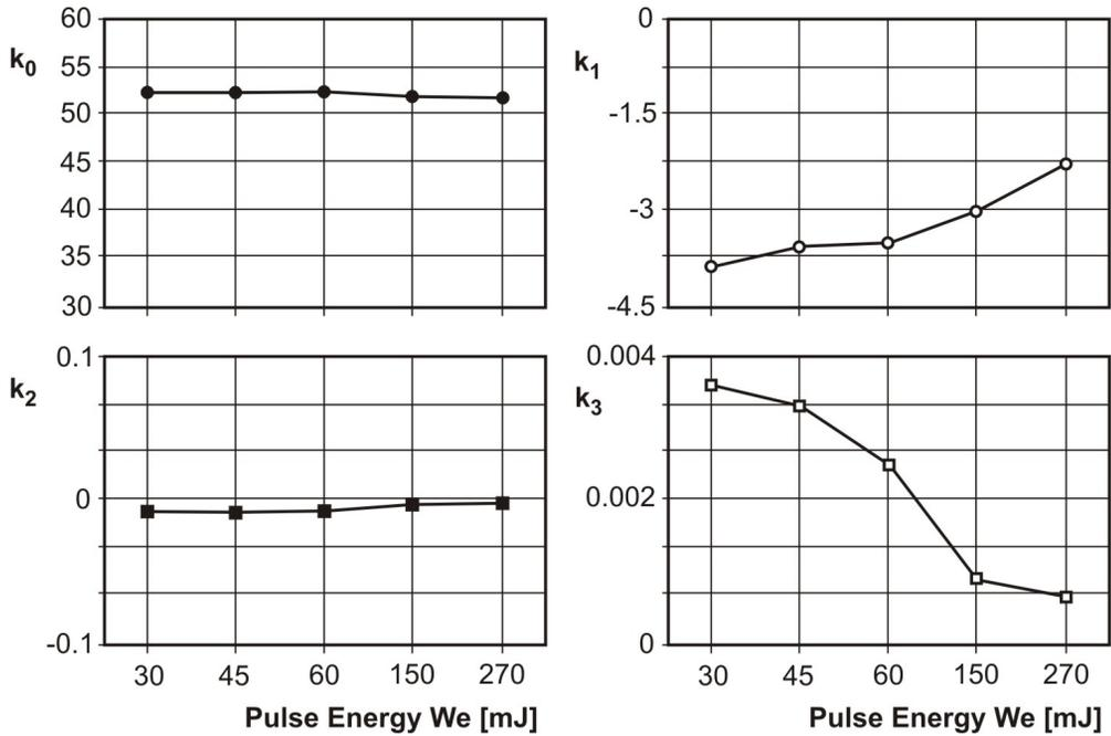
Fig. 8. Polynomial fitting coefficient against pulse energy,  $W_e$  ( $k_0$ : constant,  $k_1$ : linear,  $k_2$ : square,  $k_3$ : cubic, material: Ck 60)
