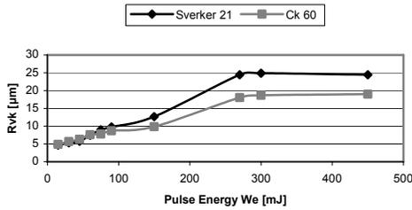
Fig. 11. Variation of  $R_{vk}$  with pulse energy,  $W_e$
