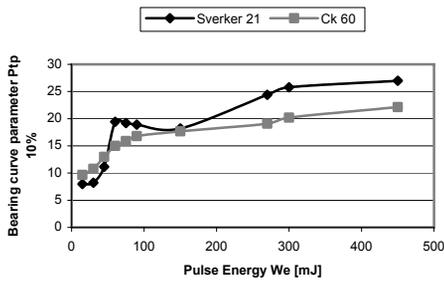
Fig. 6. Variation of  $P_{tp10\%}$  parameter of unfiltered profile with pulse energy,  $W_e$
