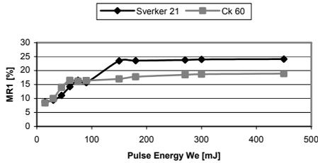
Fig. 12. Variation of  $M_{R1}$  parameter with pulse energy,  $W_e$
