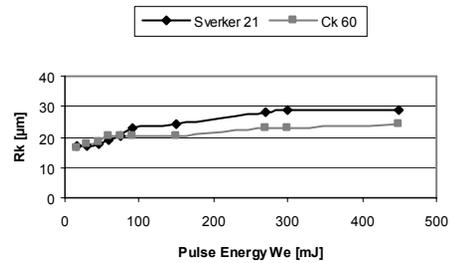
Fig. 9. Variation of  $R_k$  with pulse energy,  $W_e$
