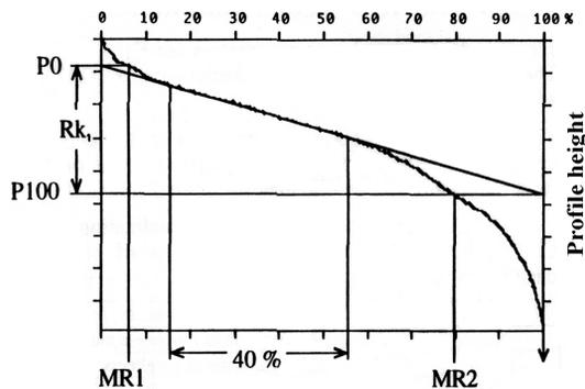
Fig. 1. Definition of the family of "R<sub>k</sub>" parameters
