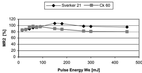
Fig. 13. Variation of  $M_{R2}$  parameter with pulse energy,  $W_e$
