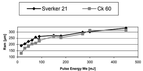
Fig. 5. Variation of the mean asperities spacing,  $R_{sm}$  with pulse energy  $W_e$ .
