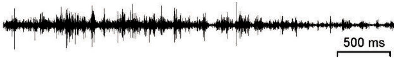
Fig. 6: Oscillogram of the vibrational signal produced by a walking mealworm beetle ( Tenebrio molitor ), when the accelerometer was buried 1 cm deep into substrate. In this experiment, coarse sand with particle sizes 1000–2200 \mu\text{m} was used.
