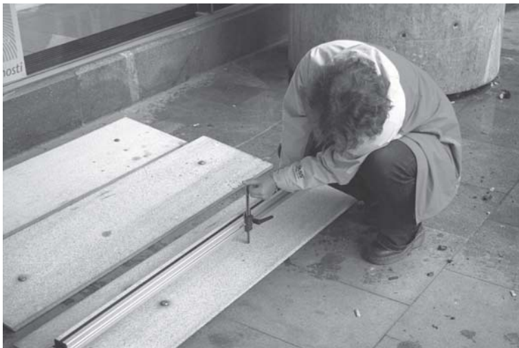
Figure 3. Bowing measurements of panels, which had been detached from the west façade
