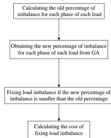
Figure 2. Flowchart of fixing the load imbalance.
