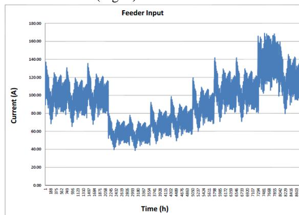
Figure 6. Load curve for the Shrif-Abad feeder input for the 12-month period under study.
