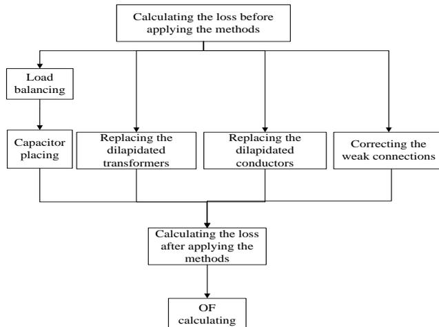
Figure 3: OF flowchart for each iteration
