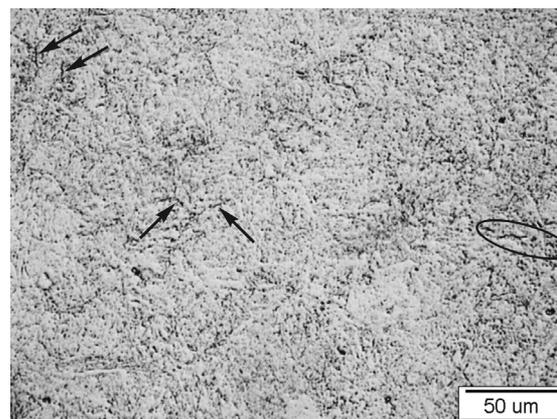
**Figure 9:** Microstructure of the HAZ in the welded joint of the T-fitting
