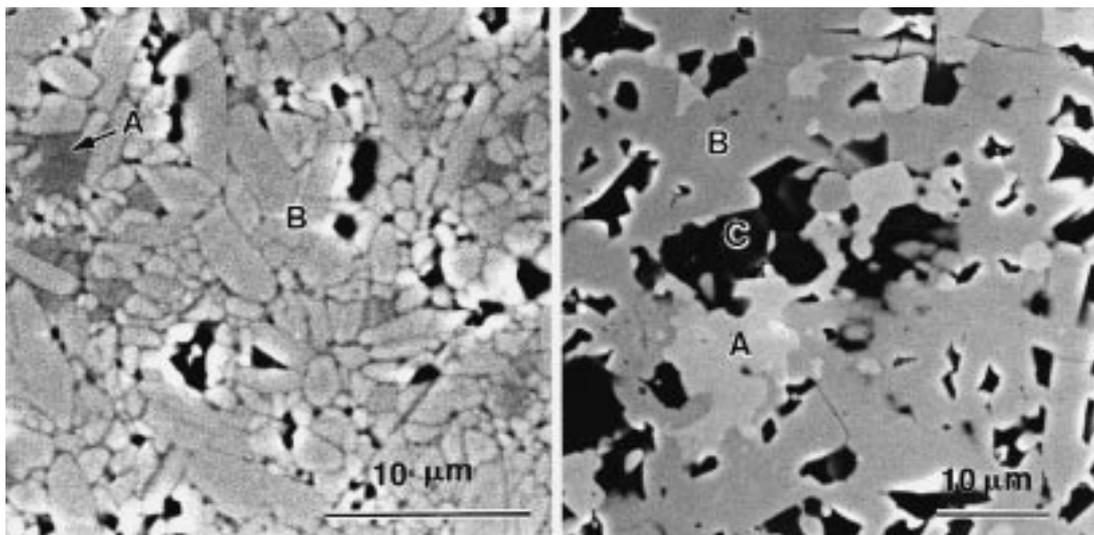
Fig. 5: Microstructure of composition  $\text{Ba}_{6-x}\text{Gd}_{8-2/3x}\text{Ti}_{18}\text{O}_{54}$  with  $x = 1.0$ .
