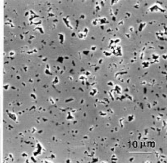
Fig. 4: Microstructure of composition Ba<sub>6-x</sub>Gd<sub>8+2/3x</sub>Ti<sub>18</sub>O<sub>54</sub> with x = 1.2. Single-phase structure.
