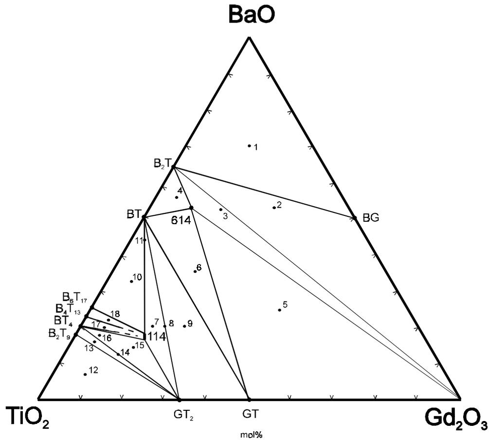
Fig. 1: Subsolidus phase diagram of the BaO-TiO<sub>2</sub>-Gd<sub>2</sub>O<sub>3</sub> system in air at 1300°C.
