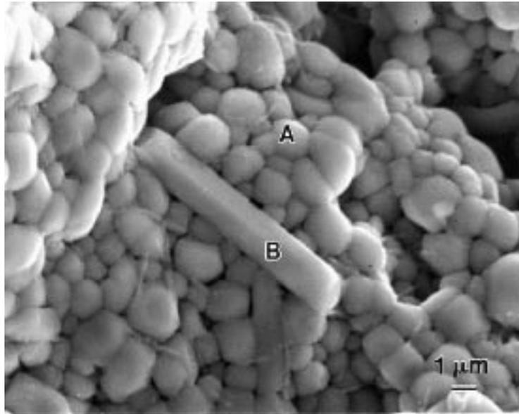
Fig. 2: Microstructure of composition 44 m/o BaO, 3 m/o Gd<sub>2</sub>O<sub>3</sub>, 53 m/o TiO<sub>2</sub> located on tie-line BT - BGT<sub>4</sub> showing the two phase structure: A = BaTiO<sub>3</sub>, B = BaGd<sub>2</sub>Ti<sub>4</sub>O<sub>12</sub>ss.
