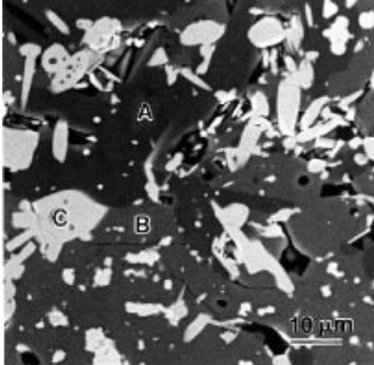
Fig. 3: Microstructure of composition 20 m/o BaO, 5 m/o Gd<sub>2</sub>O<sub>3</sub>, 75 m/o TiO<sub>2</sub> located in the compatibility triangle B<sub>4</sub>T<sub>13</sub>-114-BT<sub>4</sub> showing three phase structure: A = BT<sub>4</sub>, B = B<sub>4</sub>Ti<sub>13</sub>, C = 114.
