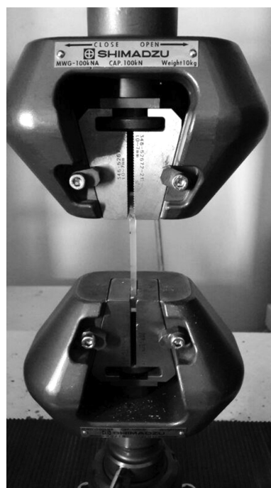
Figure 2: Specimen during the tensile test
