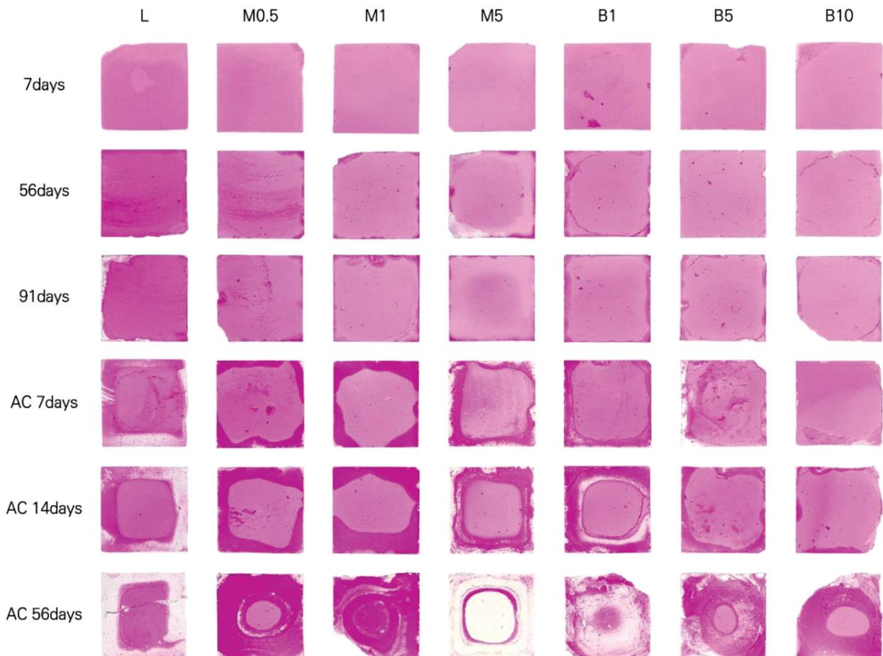
**Figure 4:** Neutralization test results (sample size of  $50 \times 50 \times 50$  mm)
