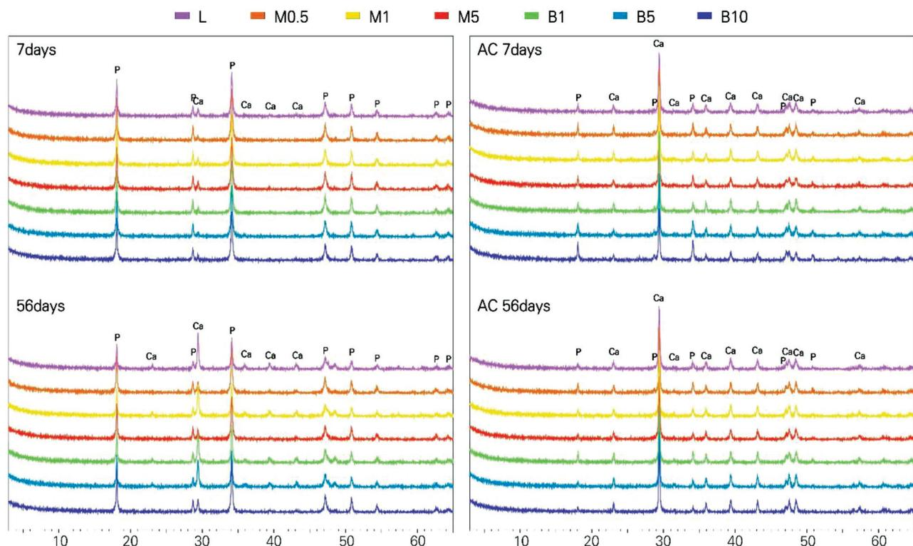
Figure 6: XRD analysis results (P – portlandite, Ca – calcite)
