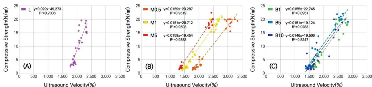
**Figure 9:** Strength correlation of lime plasters based on ultrasound velocity and compressive strength measurement: a) without perilla oil, b) with perilla oil mixed, c) with perilla oil applied
