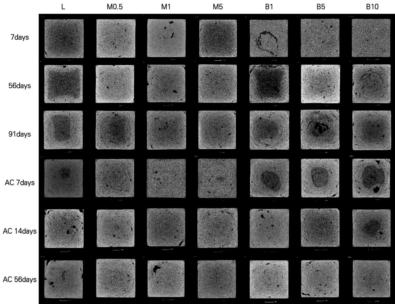
Figure 5:  $\mu$ -CT analysis images (sample size of  $(20 \times 20 \times 20)$  mm)
