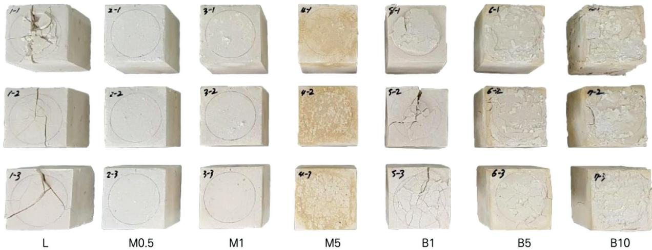
Figure 3: Freeze-thaw test results after 3<sup>rd</sup> cycle
