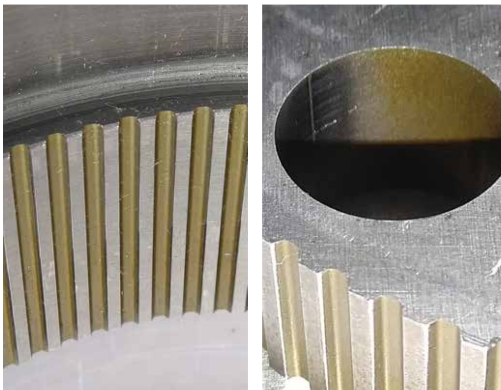
Figure 6 : Ring gear (left) and a planet (right) of a specimen 01 after disassembly.
