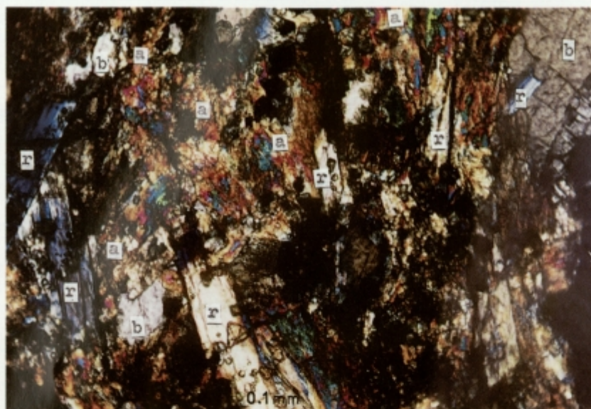
Fig. 5. Replacements of Zn-rich aegirine-augite (a) by Zn-rich richterite (r) inside of baryte (b) schist (N+, photo: S. Jančev)
