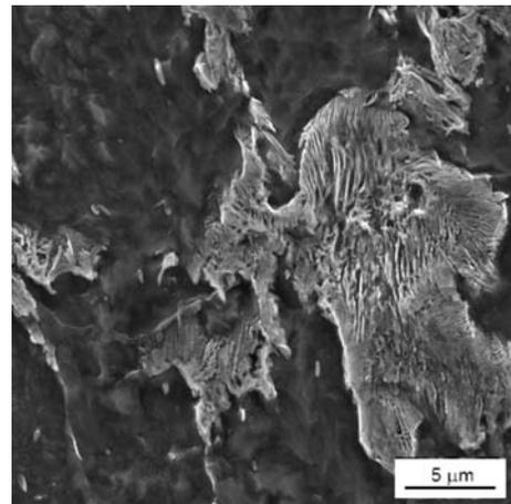
**Figure 3:** Effects of thermal cycling in the temperature range of 740–780 °C without deformation
