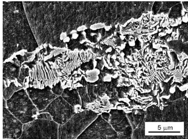
**Figure 6:** 700  $^{\circ}\text{C}/10\text{ s}$  – 5-times tension + compression ( $\varphi = 4$ ), 0 s pause between deformation cycles
