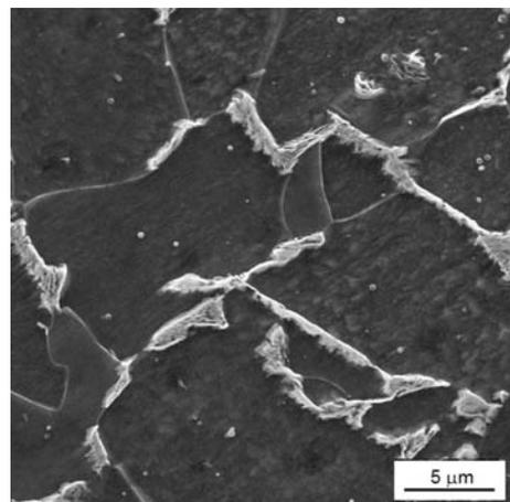
**Figure 4:** Effects of thermal cycling in the temperature range of 740–780 °C with deformation
