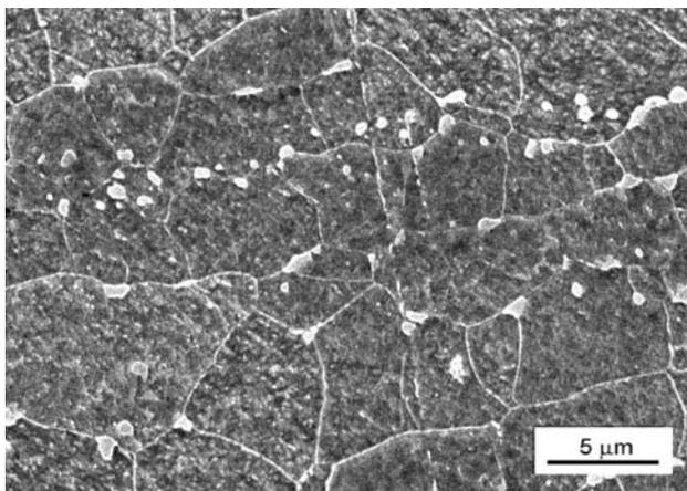
**Figure 2:** 740 °C/10 s – 2-times deformation step: tension + compression ( $\varphi = 2.1$ ) with a hold of 300 s
