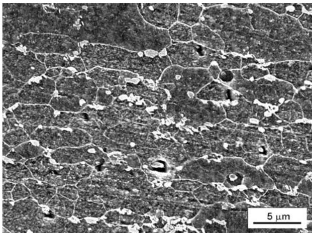
**Figure 5:** 700  $^{\circ}\text{C}/10\text{ s}$  – 9-times tension + compression ( $\varphi = 7.2$ ), 30 s pause between deformation cycles
