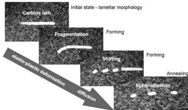
**Figure 1:** Scheme of the newly developed ASR process
