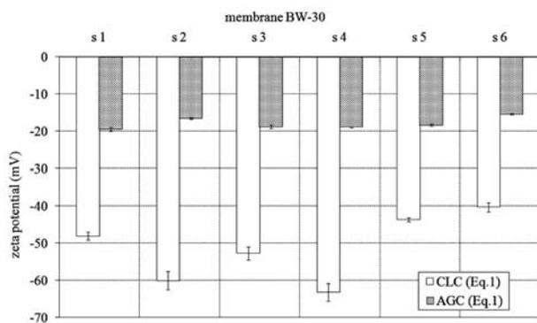
**Figure 3:** Zeta potential of membrane BW-30 obtained with “Adjustable Gap Cell” and “Clamping Cell” using Eq. 1.
