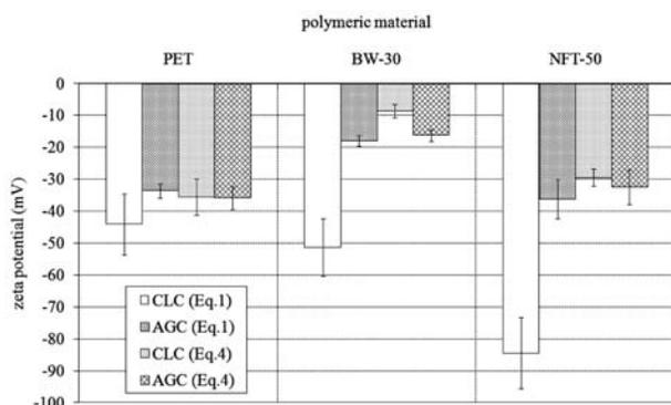
**Figure 5:** Zeta potential of selected polymeric materials obtained with AGC and CLC cells using Eq. 4 and Eq. 1
