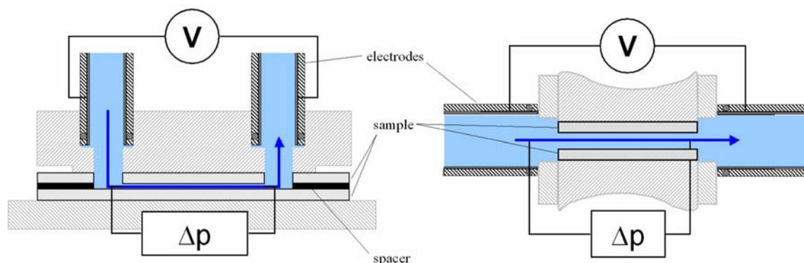
**Figure 2:** Schematic representation of tangential measuring technique in the “Clamping Cell” (left) and the “Adjustable Gap Cell” (right) of the “SurPASS” instrument.
