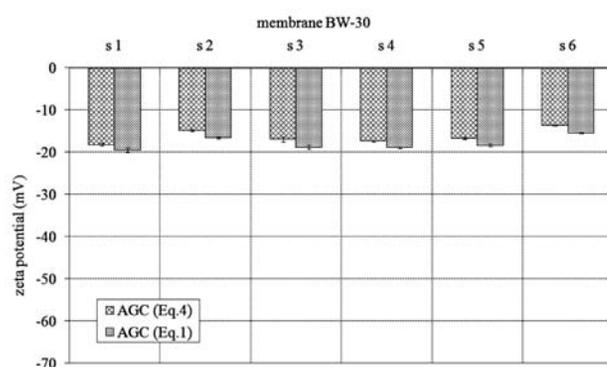
**Figure 4:** Zeta potential of BW-30 membrane obtained with “Adjustable Gap Cell” using Eq. 4 and Eq. 1.
