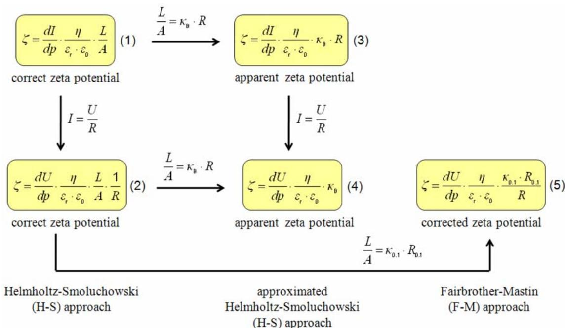
Figure 1: Different equations for zeta potential determination.
