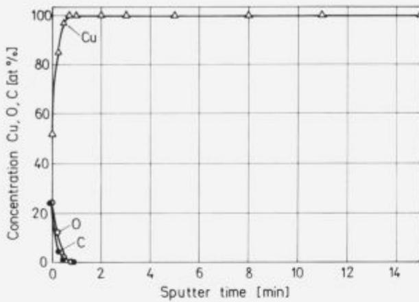
Figure 9: Copper, oxygen and carbon concentration distribution on fracture surfaces of high ductility copper (Z = 90%)
