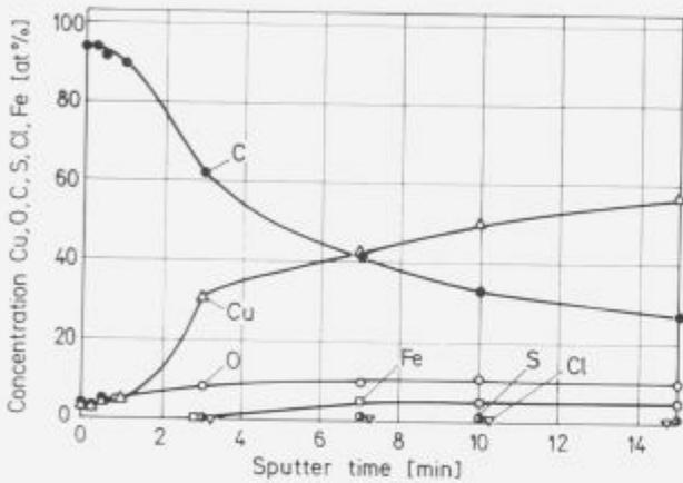
Figure 14: Oxygen, copper and other elements concentration distribution on wire surface before annealing in nitrogen
