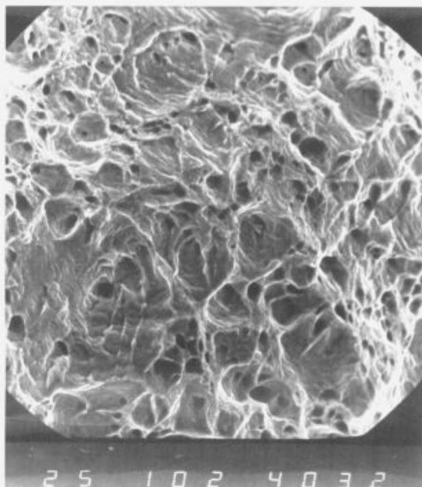
Figure 7: Ductile fracture of copper wire ( $Z = 90\%$ ); 1000x
