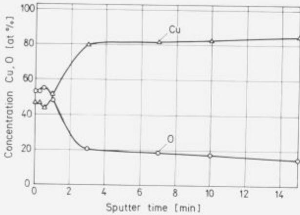
Figure 13: Copper and oxygen distribution on wire surface before annealing in nitrogen
