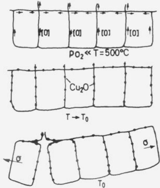
Figure 15: Mechanism sequences of copper wire embrittlement
