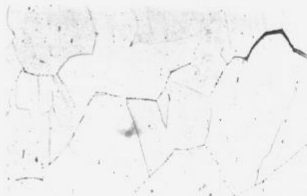
Figure 5: Small cracks on grain boundaries and copper oxide precipitates; 200x
