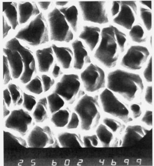
Figure 4: Detail of intergranular rupture surface with copper oxide inclusions in dimples (fig.3); 6000x
