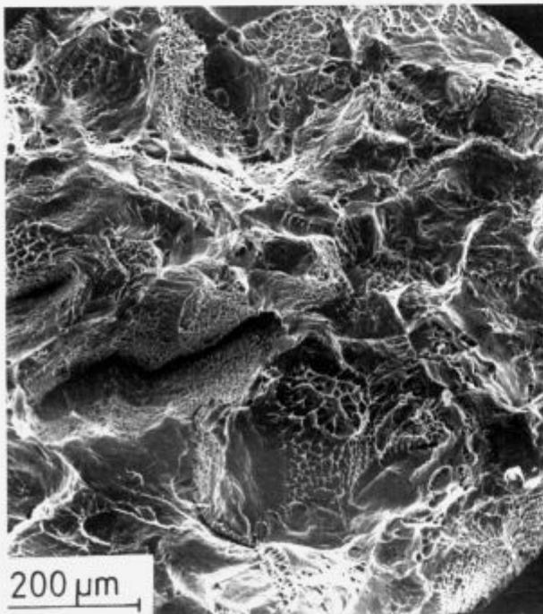
Figure 2: Intergranular dimple rupture in copper wire resulting from microvoids coalescence at grain boundaries; 100x
