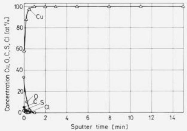
Figure 11: Copper, oxygen and other elements concentration distribution on fracture surface of copper after vacuum annealing (fracture after annealing)
