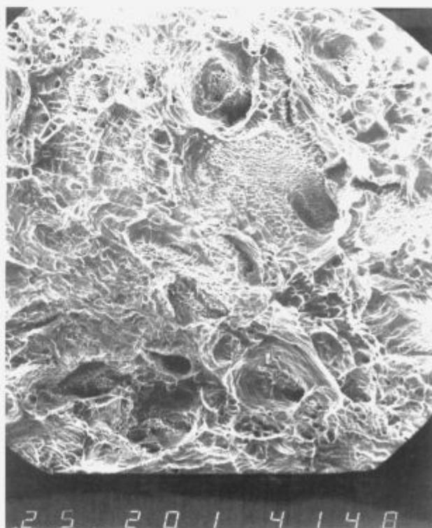
Figure 8: Fracture surface of copper wire after vacuum annealing ( $Z = 90\%$ ); 200x
