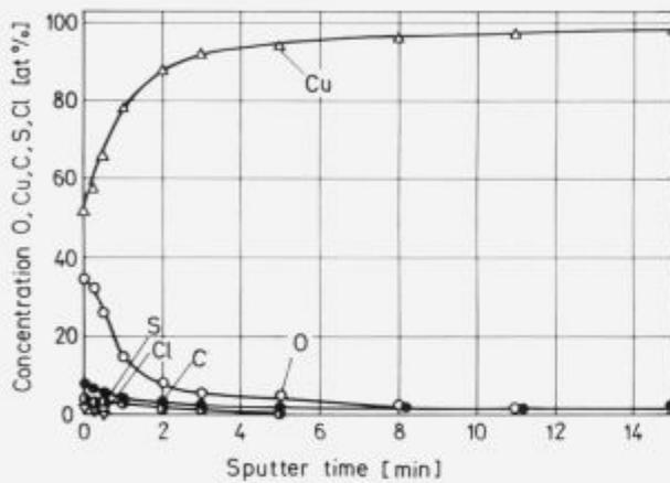
Figure 10: Copper and oxygen concentration distribution on fracture surface of copper after annealing in nitrogen (5 ... 6 ppm O<sub>2</sub>)
