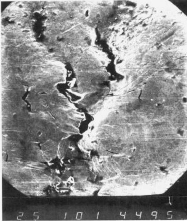
Figure 1: Cracks on copper wire surface after cold rolling (first step of reduction); 100x
