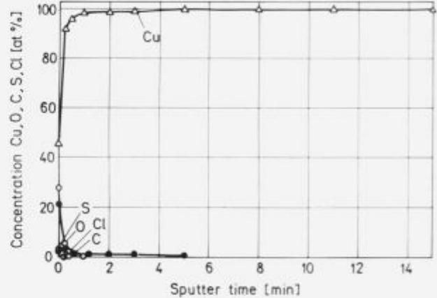
Figure 12: Copper, oxygen and other elements distribution on fracture surface after vacuum annealing (fracture before annealing)
