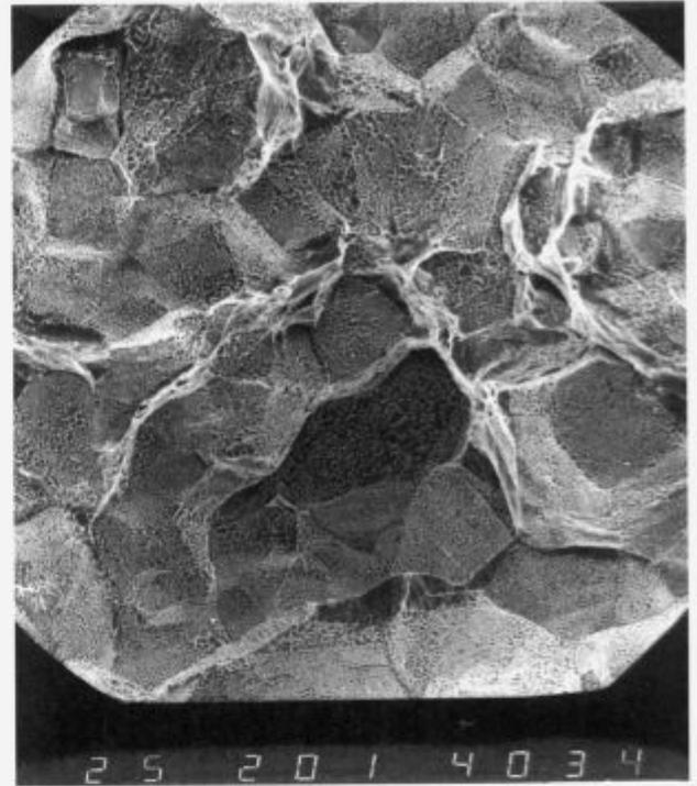
Figure 3: Intergranular dimple rupture in copper wire resulting from microvoids coalescence at grain boundaries ( $Z = 25\%$ ); 200x
