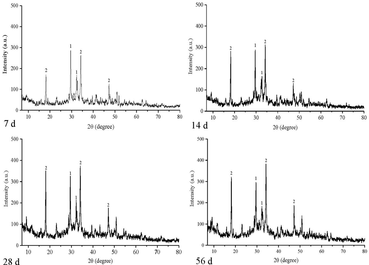
Figure 3: XRD diffraction analysis of EPCM surface cement (Note: 1 = calcium carbonate; 2 = calcium hydroxide)
