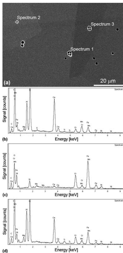
**Figure 6:** EDX spot analysis, (a) SE image of stem specimen with marked spots of EDX analysis, (b), (c) and (d) EDX spot analysis of non-metallic inclusions
