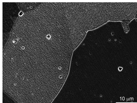
**Figure 9:** SE image of stem microstructure consist of austenite grains. Grain boundaries are free of any carbides and other phases. Etched by glyceric acid
