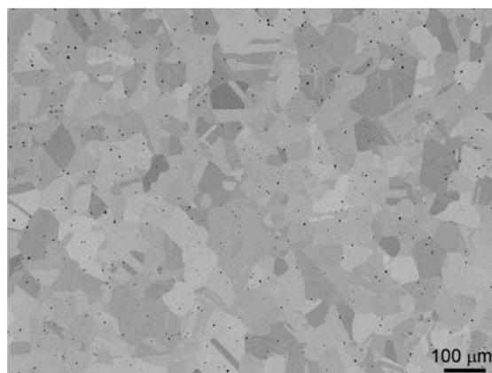
**Figure 5:** Microstructure of stem specimen showing plenty of  $Al_2O_3$  non-metallic inclusions, BE image
