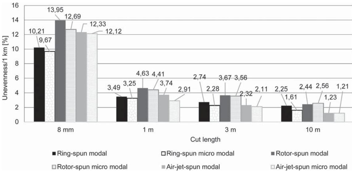
Figure 2: Unevenness of ring-, rotor- and air-jet-spun modal and micro modal yarns at different cut lengths
