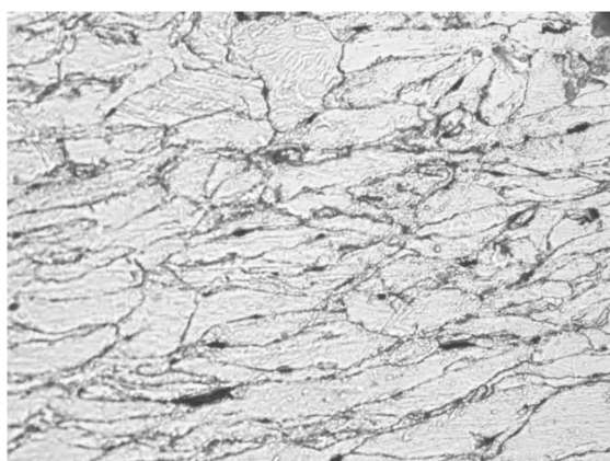
Figure 5: Microstructure of the as-rolled composite with 1.0 % of mass fraction of graphene content after the aging time of 3 h
