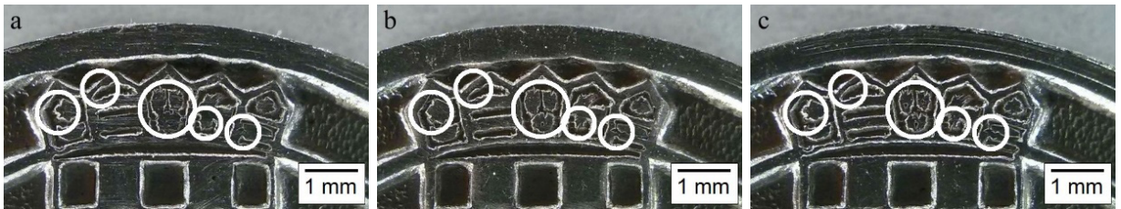
Fig. 5. Geometry details of the coin with different crystalline grain size a) 25 \mu\text{m} , b) 50 \mu\text{m} , c) 90 \mu\text{m} , obtained with 150 kN forging force
