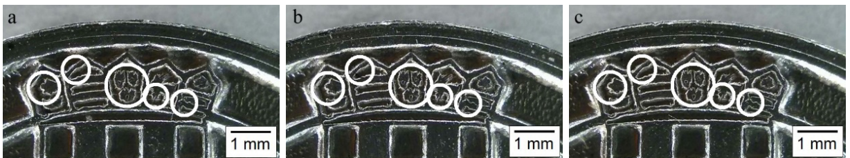
Fig. 6. Geometry details of the coin with different crystalline grain size a) 25 \mu\text{m} , b) 50 \mu\text{m} , c) 90 \mu\text{m} , obtained with 200 kN forging force
